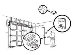
1. Press the Prog < Learn > button on the LCD/Motion Detecting Control Console.
