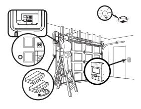
1. Press and release the purple "learn" button on the motor unit. The learn indicator light will glow steadily for 30 seconds.
