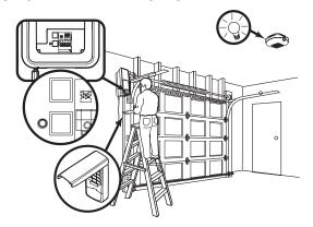
Press and release the purple "learn" button on motor unit. The learn indicator light will glow steadily for 30 seconds.
