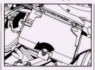
Remove the nut on the outboard side of the unit. Then loosen the front and inboard nuts. For the LT5 engine, loosen the two inboard nuts. Move the ECM unit to either side.
