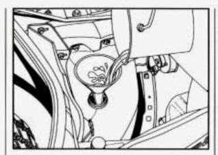
Then fill the coolant recovery tank to the "HOT" mark on the dipstick.
