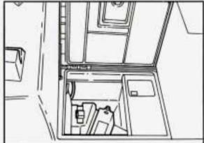
The jack, wheel nut socket and wheel lock key are in the rear storage compartment behind the passenger's seat. Open the compartment door and remove the plastic tray. Lift the jack, wheel nut socket and wheel lock key out of the foam
