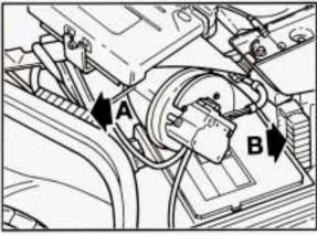
The other two fuse blocks are in the engine compartment. One is part of the Forward Lamp wiring harness (A), and the other is part of the ECM-Engine wiring harness (B).
