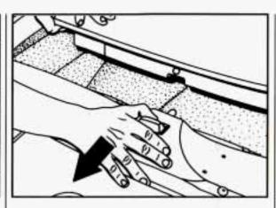
Store the roof panel with its top up and its rear pointing forward. Slide the rear corners of the roof panel into the brackets and push forward.
