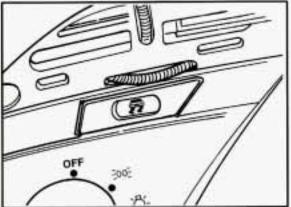
The ASR system automatically comes on whenever you start your vehicle. To limit wheel spin, especially in slippery road conditions, you should always leave the system on. But you can turn the ASR system off if you ever need to. (You should turn the system off if your vehicle ever gets stuck in sand, mud, ice or snow. See "Rocking Your Vehicle" in the Index.)
