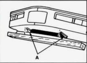
Position 4x4 wood beam across sling chains contacting under fascia just ahead of curb protect brackets (A).
