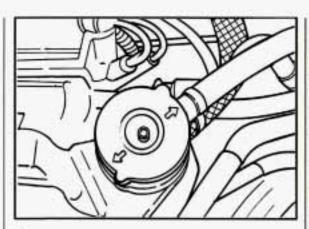
8. Shut the engine off and replace the pressure cap. At any time during this procedure if coolant begins to flow out of the filler neck, reinstall the pressure cap. Be sure the arrows on the cap line up like this.
