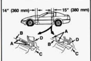
Position the jack under the vehicle. There are two locator triangles (A) on the panels (B) near each wheel. Raise the lift head (C) until it fits firmly under the steel rocker flange (D) between the triangles nearest the flat tire.
