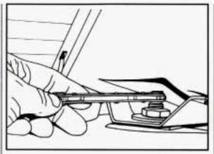
Loosen the rear corner bracket bolts with the ratchet.
