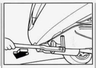
The spare tire is on a tire carrier tray under the rear end of your vehicle. To lower the tray, use the socket end of the wheel wrench to turn the latch bolt counterclockwise. Lower the tray about an inch. Don't loosen the latch bolt too much, or the tray could fall.
