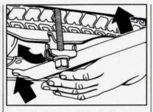
Put the hooked end of the wheel wrench into the slot in the tray. Lift the tray using the wheel wrench and insert the latch bolt into the notch in the tray. To raise the tray, use the socket end of the wheel wrench to turn the latch bolt clockwise. Turn the latch bolt until it is snug.
