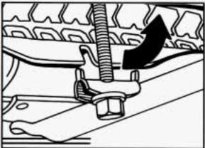
While holding the tray up with the wheel wrench, pull the latch bolt to release it from the tray. If it won't come free, loosen it a little more.
