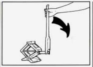
Attach the wheel wrench to the jack. Hold the wheel wrench handle so it forms a right angle with the jack, then turn it clockwise.
