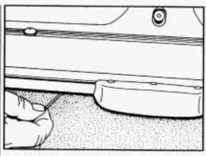
If you don't have battery power, use the manual release cable to open the hatch. The cable is near the security shade handle, between the carpet and the shade.
