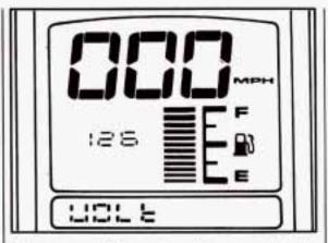
If you must drive a short distance with the voltmeter reading in a shaded area, turn off all your accessories, including your comfort controls and audio systems.
