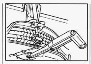
Put the hooked end of the wheel wrench into the slot in the tray. Insert the wheel wrench a little from the side so it isn't over the latch bolt. Pull up on the wheel wrench to lift the tray.
