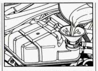
Fill the coolant high fill reservoir with the proper mix, up to the base of the filler neck.
