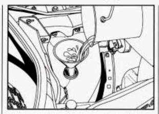
If you need to add more coolant, add the proper mix at the coolant recovery tank, but only when your engine is cool. If the tank is very low or empty, also add coolant to the coolant high fill reservoir. See "Engine Overheating" in the Index for information.
