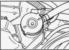
Shut the engine off and replace the pressure cap. Be sure the arrows on the pressure cap line up like this.
