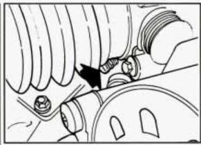
After the engine cools, open the air bleed valves on the throttle body. . .
