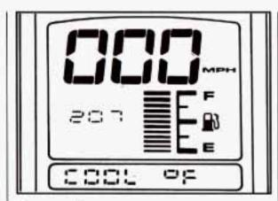
For numeric gauge measurements, press the "GAUGES" button on the Trip Monitor until "COOL" appears. The number that appears next to the fuel gauge is the coolant temperature. If "LO" appears, the temperature is below 32°F (0°C).
