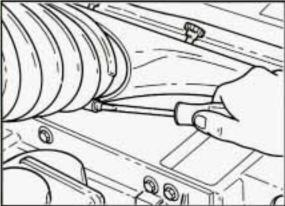
Disconnect the clamp from the manifold.
