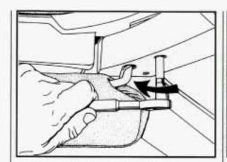
Loosen the front bolts with the wrench.
