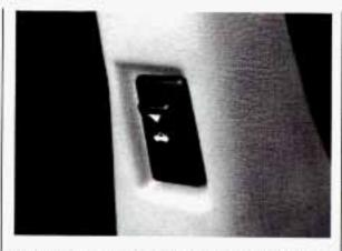
If you have a coupe, this switch is on the rear of the driver's door. It works with the door open and the transmission in any gear. Push it down to release the hatch.
