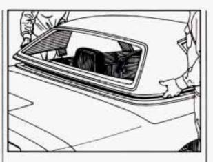
10. With one person on each side, gently lift the hardtop about eight inches (200 mm) straight up. Remove the hardtop over the rear of the vehicle.
