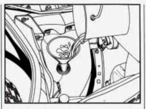
Then fill the coolant recovery tank to the proper level.
