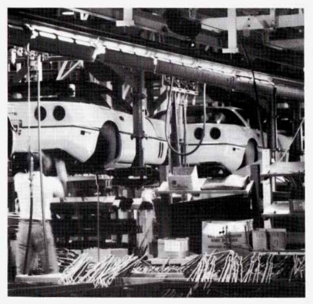
The Corvette Assembly Plant in Bowling Green, Kentucky, is one of the most sophisticated and computerized automobile assembly facilities in the world. To build your 1994 Corvette, over 1,200 employes teamed up with the 70 high-tech robots that assist in a variety of processes, from welding to painting.
