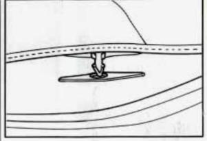
Lower the rear of the top so the latch pins align with the holes in the lid. To secure the rear of the top, push down firmly on both corners.
