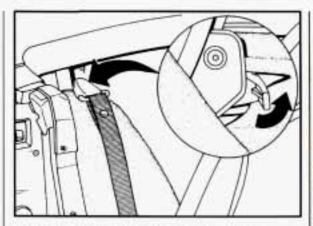
If your Corvette has lost power (dead battery, for example), you can still open the storage compartment using the manual release handles. The handles are near the sidewall behind the safety belt anchors on each side of your vehicle. Move the handles toward the rear of the vehicle and upward.
