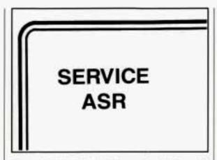
The "SERVICE ASR" warning light will come on to let you know if there's a problem with the ASR system. See "ASR System Warning Light" in the Index. When this warning light is on, the system will not limit wheel spin. Adjust your driving accordingly.
