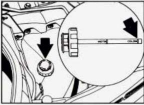
If the coolant inside the coolant recovery tank is boiling, don't do anything else until it cools down.
