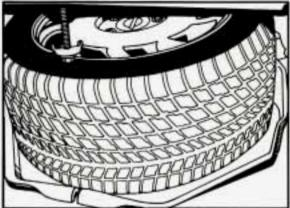
Put the flat road tire on the tray. Lift the latch bolt, push it toward the front of the vehicle, and the bolt will drop down to the lower position.
