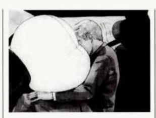
The right-front passenger's air bag is located in the instrument panel on the passenger's side.
