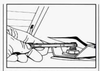
Secure but don't tighten the rear corner bracket bolts using the ratchet.
