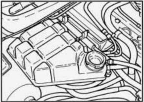
Put the cap back on the coolant recovery tank, but leave the coolant high fill reservoir pressure cap off.
