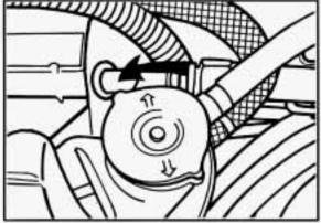
How to Add Coolant to the Coolant High Fill Reservoir – LT1 Only
