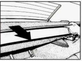
Move both seatbacks forward and remove the rear trim panel.
