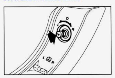
The electric mirror control is on the driver's door. To adjust either mirror, turn the switch to LEFT (L) or RIGHT (R). Then use the control to adjust the mirror. When you are done adjusting the mirrors, move the control back to the center to avoid accidental adjustment.
