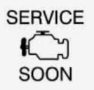
Your Corvette is equipped with a computer which monitors operation of the fuel, ignition and emission control systems.
