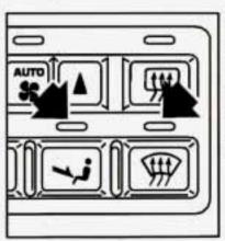
To turn on DEFOG, push the HEATER and DEFROST buttons at the same time. Both green lights above the buttons will come on to let you know that DEFOG is working.
