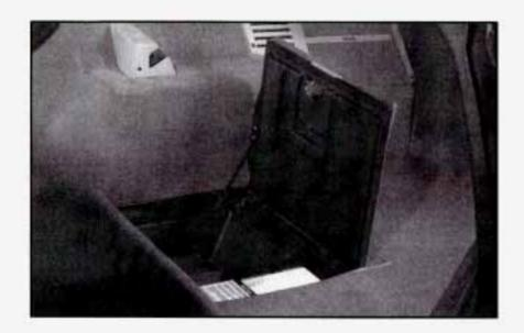
The jack, wheel nut socket and wheel lock key are in the rear storage compartment behind the passenger's seat.
