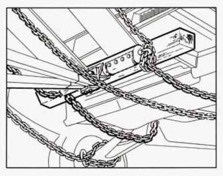
Position the sling crossbar against the front of the  $4'' \times 4''$  beam.
