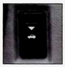
If you have a coupe, this switch is on the rear of the driver's door. It works with the door open and the transmission in any gear. Push it down to release the hatch.
