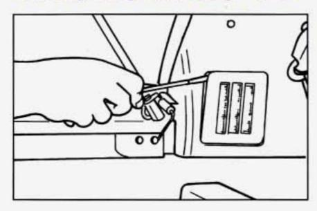
Pry the cover off with a screwdriver. Be sure to pry from the rear side, or you could break the tab on the cover.
