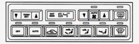
With this system, you set a temperature and then either let the system adjust airflow and force to maintain the temperature, or you can manually adjust flow and force.
