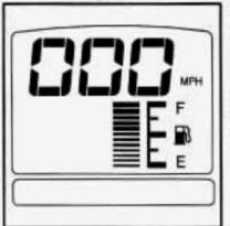
Your fuel gauge shows about how much fuel is in your tank. The bars light up when the ignition is on or, if the ignition is off, when you turn on your parking lamps.
