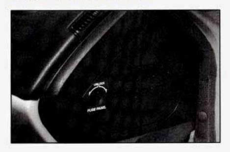
The interior fuse center is on the right side of your instrument panel. Turn the knob and pull the door to access the fuses.
