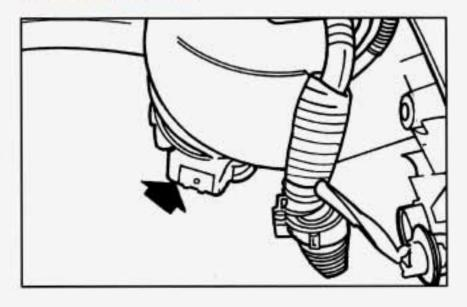
You can reach the front cornering lamp from inside the engine compartment.
