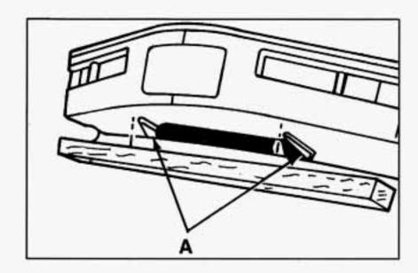
Position a  $4'' \times 4''$  wood beam across sling chains contacting under fascia just ahead of the curb protect brackets (A).
