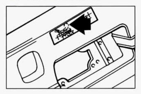
You can reach the center high-mounted stoplamp by removing the license plate and reaching through the opening.
