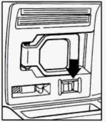
Push the power door lock switch on either door backward to lock or forward to unlock both doors at once.
