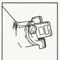
If you have a manual transmission, your ignition lock has a key release button. You must press the button before you can take your key out of the ignition lock.
