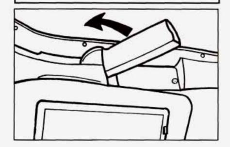
Unlock the front of the convertible top by turning the latch handles outward. Then lift the top off the windshield slightly.
