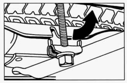
While holding the tray up with the wheel wrench, pull the latch bolt rearward to release it from the tray. If it won't come free, loosen it a little more.
