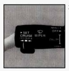
Push in the SET button at the end of the lever and release it.
