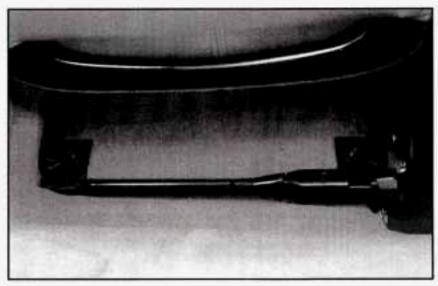
The wheel wrench is on the floor behind the driver's seat. Move the driver's seat all the way forward and fold the seatback forward. Loosen the wingnuts and slide the wheel wrench out of the clamps.
