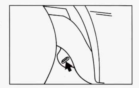
Attach T-hook chains on both sides into slotted holes behind and inboard of the front wheels. Use these slots for sling equipment and car carrier securing.
