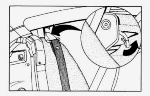
6. If your Corvette has lost power (dead battery, for example), you can still open the storage compartment using the manual release handles. The handles are near the sidewall, behind the safety belt anchors on each side of your vehicle. Move the handles toward the rear of the vehicle and upward.
