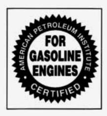
Oils meeting these requirements should also have the "Starburst" symbol on the container. This symbol indicates that the oil has been certified by the American Petroleum Institute (API). Do not use any oil which does not carry this Starburst symbol.
