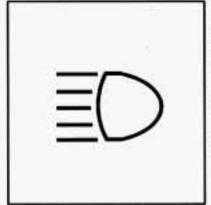
To change the headlamps from low beam to high or high to low, pull the turn signal lever all the way toward you. Then release it. When the high beams are on, this light on the instrument panel also will be on.
