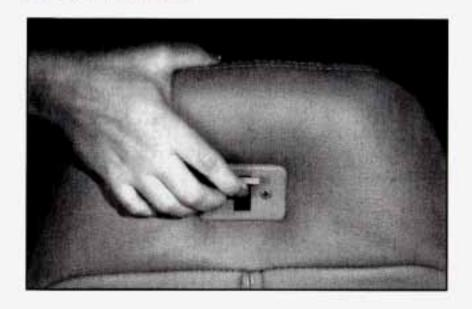
Both scatbacks fold forward to give you access to the rear area. To fold a seatback forward, lift this latch and push the seatback forward. When you return the seatback to its original position, make sure the seatback is locked.
