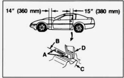
When you've turned the wrench almost as far as it will go, swing it around to the other side. Keep turning to raise the jack lift head a 3 inches (76.2 mm).  Position the jack under the vehicle. There are two locator triangles (A) on the panels (B) near each wheel. Raise the lift head (C) until it fits firmly under the steel rocker flange (D) between the triangles nearest the flat tire.
