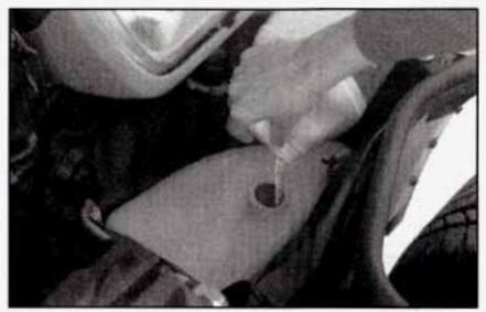
10. Then fill the coolant recovery tank to the proper level.
