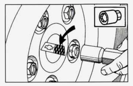
Each wheel will have one locknut. A special wheel lock key (removal tool) and instructions are provided. Attach the wheel lock key to the wheel wrench. Remove the locking wheel nut by turning counterclockwise.
