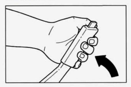
To set the parking brake, hold the brake pedal down. Pull the parking brake lever up, then move it back down. This sets your parking brake, even though the lever is down. If the ignition is on, the parking brake indicator light will come on.
