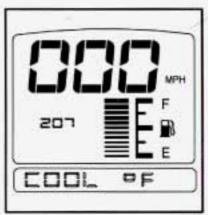
For numeric gauge measurements, press the GAUGES button on the trip monitor until COOL appears.
