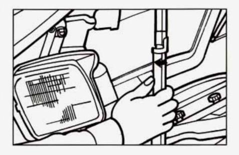
Then release the hood strut by moving it to the centered position and lowering the hood. Lower the hood until the bottom of the hood is the same height as the top of the windshield, then release it.
