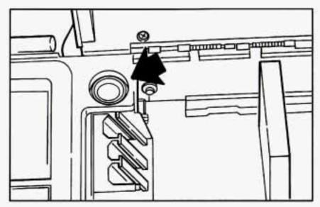
Press the switch in your center console to unlock the hatch from inside your vehicle. If you have an automatic transmission, your shift lever must be in PARK (P) or NEUTRAL (N) to use the switch. If you have a manual transmission, you must set the parking brake before you can use the switch when the vehicle is running. If you have a manual transmission and the vehicle is not running, you may use the switch in any gear.
