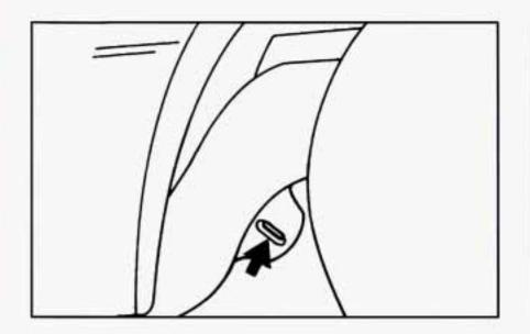
Attach T-hook chains in slots forward and just inboard of the rear wheels on both sides.
