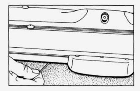
If you don't have battery power, use the manual release cable to open the hatch. The cable is near the security shade handle, between the carpet and the shade.
