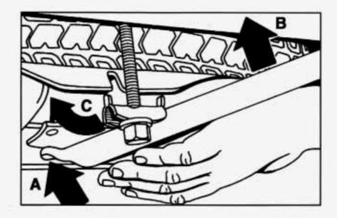
Put the hooked end of the wheel wrench into the slot in the tray (A). Lift the tray using the wheel wrench (B) and insert the latch bolt into the notch in the tray (C). To raise the tray, use the socket end of the wheel wrench to turn the latch bolt counterclockwise. Turn the latch bolt until it is snug. Put the wheel wrench back in its place under the driver's seat. Be sure to tighten the wingnuts.
