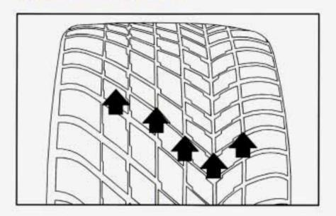
One way to tell when it's time for new tires is to check the treadwear indicators, which will appear when your tires have only 1/16 inch (1.6 mm) or less of tread remaining.
