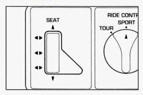
If you have the Sport Seat, you must move the switch next to the lumbar controls to DR (driver) or PS (passenger) before adjusting your power seat. Different parts of the power seat control move different parts of your seat. If you move the whole control, the whole seat will move. The back of the control will move the back of the seat, and the front of the control will move the front of the seat.
