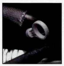
The engine oil dipstick is next to the coolant high fill reservoir. The dipstick handle is a round, yellow loop.
