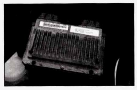
You must loosen and remove the two screws before the PCM unit will lift out. Fluid should be added if the fluid level is at or below the ADD mark on the reservoir. There are additional instructions on the reservoir cap.
