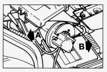
There are two maxi-fuse blocks in the engine compartment. One is part of the forward lamp wiring harness (A), and the other is part of the ECM-engine wiring harness (B).
