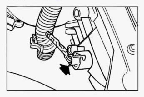
You can reach the front sidemarker lamp from inside the engine compartment.
