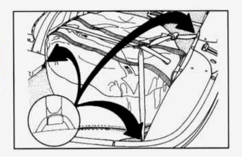
A Grand Sport Coupe rear tire will not fit in the tray, so you must put in on the floor of the rear area. Put the flat tire in the storage bag provided with the spare. Place the tire on the rear area floor.
