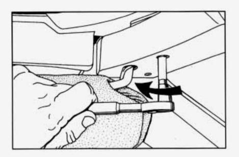
2. Loosen the front bolts with the wrench.
