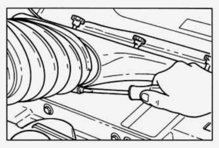
2. Disconnect the clamp from the manifold.
