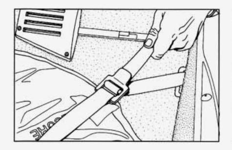
When the tire is stored in the rear cargo area, you can't store a removable roof panel. It will not fit into the latches properly. Raise the tire carrier tray to its upper position and tighten the latch bolt until it is snug.
