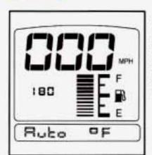
Automatic transmission fluid temperature will be displayed if you press the GAUGES button on the trip monitor until AUTO appears.
