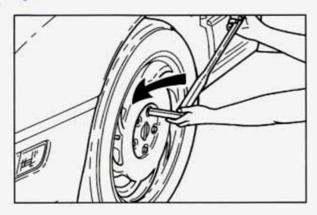
Remove the plastic wheel nut caps using the socket end of the wheel wrench by turning the wrench in the direction shown. Store the caps somewhere until you have the flat tire repaired or replaced.
