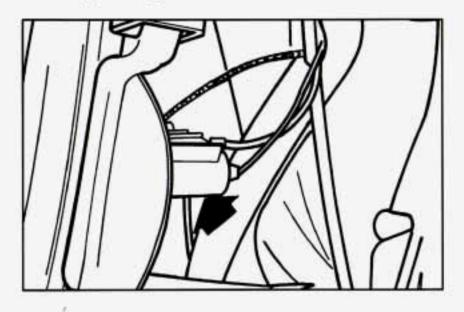
You can reach the back-up lamps by removing the license plate and reaching through the opening.
