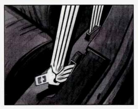
If you do not want the lap belt to move freely, push the CINCH button. To loosen the belt, unbuckle it, let it retract, and buckle up again.
