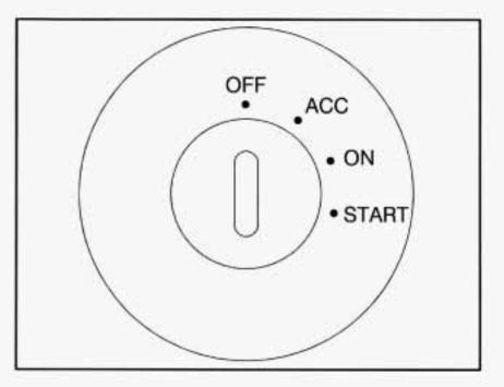
With the key in the ignition switch, you can turn the switch to four positions. **OFF:** The only position from which you can remove the key. Removing the key locks your steering wheel, ignition and automatic transmission.
