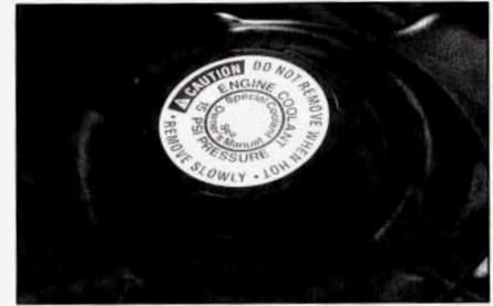
Then replace the pressure cap. Be sure the pressure cap is tight.
