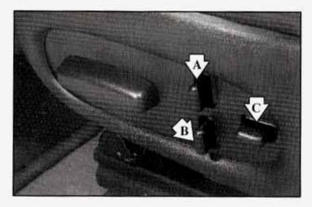
In addition to the power seat control, there are three other switches that help you change the shape of your seat. There are two lumbar supports (A and B) for the middle and lower back. There's also a side bolster switch (C) that adjusts the sides of the seat around you to give you more lateral support.
