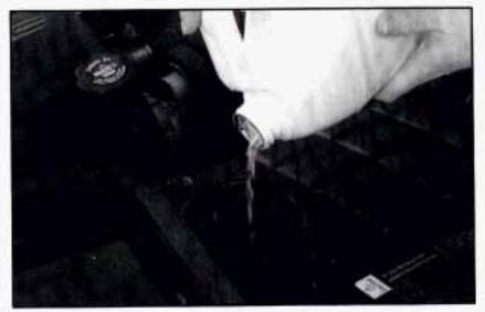
Then fill the coolant surge tank with the proper mix, up to the FULL COLD mark.
