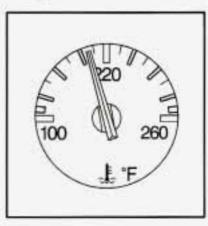
This gage shows the engine coolant temperature. If the gage pointer moves into the shaded area, your engine is too hot!
