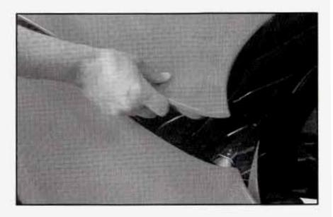
Then go to the side of the vehicle and pull up on the rear edge of the hood, near the windshield. You'll see the following when you open the hood:
