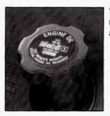
The engine oil fill cap is on top of the right valve rocker arm cover.
