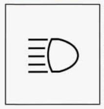
To change the headlamps from low beam to high or high to low, push the turn signal lever all the way forward. When the high beams are on, this light on the instrument panel also will be on. To change the headlamps from high to low, pull the lever rearward.
