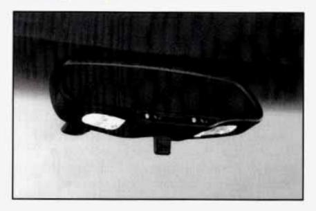
Your inside rearview mirror includes two reading lamps. The lamps will go on when a door is opened. When the doors are closed and the ignition is on, each lamp can be turned on individually by moving the switch (each lamp has its own switch) to ON.
