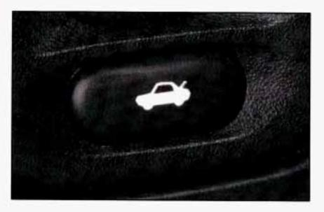
Press the button with the trunk symbol on it, at the left side of the steering column on the instrument panel, to release the hatch from inside your vehicle.
