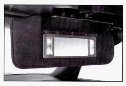
Pull down the sun visor and lift the cover to expose the vanity mirror. When the cover is lifted, the lights will come on automatically, even if the ignition is off.
