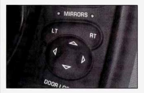
The electric mirror control is on the driver's door. To adjust either mirror, press the LT (left) or RT (right) switch to select the mirror, then press the arrows to adjust the direction of the mirror. The selected mirror will stay on for 20 seconds after the last adjustment. An indicator light will come on above the mirror that you select.
