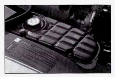
The coolant surge tank is in the engine compartment behind the headlamp on the passenger's side.
