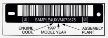
This is the legal identifier for your Corvette. It appears on a plate in the front corner of the instrument panel, on the driver's side. You can see it if you look through the windshield from outside your vehicle. The VIN also appears on the Vehicle Certification and Service Parts labels and the certificates of title and registration.
