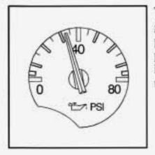
The engine oil pressure gage shows the engine oil pressure in psi (pounds per square inch) or kPa (kilopascals) when the engine is running.
