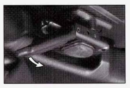
4. To unlock the front of the roof panel, pull down each of the front handles. Grasp the handles with your fingers and pull each toward you. Complete a 180° rotation toward the center of the vehicle. Then push up on each of the handles.
