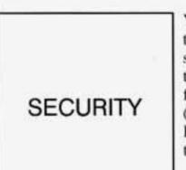
Your Corvette has a theft-deterrent alarm system. With this system, the SECURITY light will flash as you open the door (if your ignition is off). This light reminds you to arm the theft-deterrent system.
