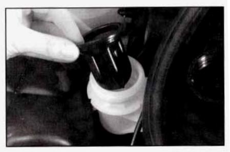
Fluid should be added if the fluid level is below the step on the inside of the reservoir. There are additional instructions on the reservoir cap.
