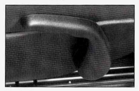
The lever for the reclining seat back is located on the side of each seat, near the base.
