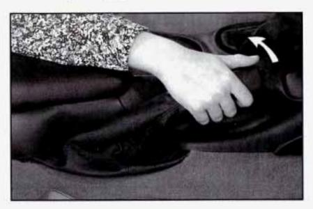
To set the parking brake, hold the brake pedal down. Pull the parking brake lever. This sets your parking brake. If the ignition is on, the brake system warning light will come on.
