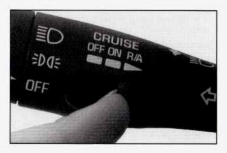
Once you're going about 25 mph (40 km/h) or more, you can move the cruise control switch to R/A (Resume/Accelerate) for about half a second. The DIC will display the cruise set speed.
