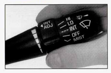
You can control the windshield wipers by moving the lever with the wiper symbol on it. This lever is located on the right side of your steering column.
