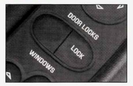
Press the power door unlock/lock switch on either door to lock or unlock both doors at once.
