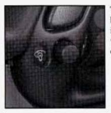
This button controls the brightness of your instrument panel lights when your headlamps or parking lamps are on.
