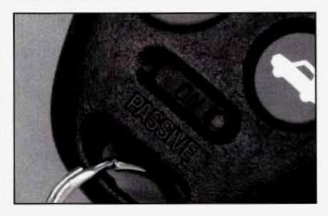
You can turn on the passive feature by moving the transmitter's slider switch to ON. Now, when you move toward your vehicle with the key fob transmitter, the system will automatically disarm your theft-deterrent system and unlock the doors. If it's dark enough outside, your interior lamps will come on. You can also use the buttons on the transmitter to actively unlock your vehicle. Press UNLOCK once to unlock the driver's door, or press UNLOCK again within 10 seconds to unlock both doors.
