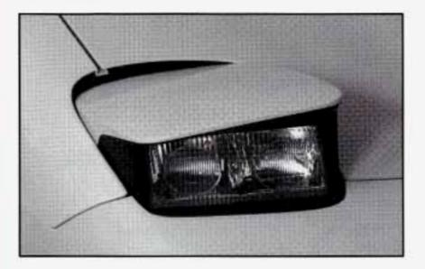
The headlamp doors are designed to open when you turn the headlamps on, and close when you turn the headlamps and parking lamps off. The headlamp doors will stay open if the headlamps are on and then the headlamp switch is turned back to the parking lamps setting. You can open the doors manually using the knob next to the headlamp assembly. Turn the knob to the left until the doors are open.
