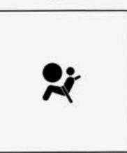
This light will come on when you start your engine, and it will flash for a few seconds. Then the light should go out. This means the system is ready.
