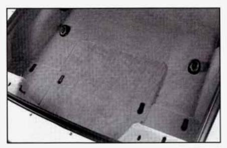
There are three rear storage compartments in the floor of the rear hatch area.
