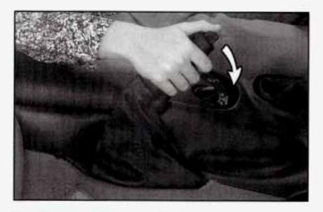
To release the parking brake, hold the brake pedal down. Hold the release button in as you move the brake lever all the way down.
