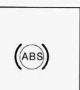
With the anti-lock brake system, the light will come on when you start your engine and may stay on for several seconds. That's normal.
