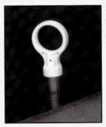
The engine oil dipstick is next to the coolant surge tank. The dipstick handle is a round, yellow loop.
