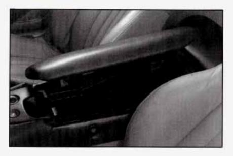
To use this storage area, pull up the lid on the driver's side front edge of the console and swing it to the passenger's side.
