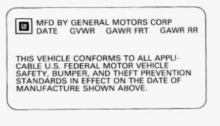
The other label is the Certification label, found on the rear edge of the driver's door. It tells you the gross weight capacity of your vehicle, called the GVWR (Gross Vehicle Weight Rating). The GVWR includes the weight of the vehicle, all occupants, fuel and cargo. Never exceed the GVWR for your vehicle, or the GAWR (Gross Axle Weight Rating) for either the front or rear axle.
