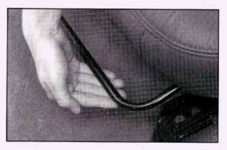
Pull up on the lever in front of the seat to unlock it.
