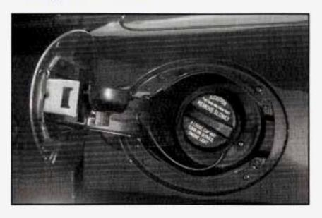
The fuel filler door is on the driver's side of the vehicle. The fuel cap is attached by a tether for your convenience.
