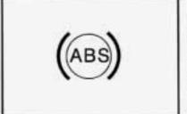
With the anti-lock brake system, the light will come on when you start your engine and may stay on for several seconds. That's normal.
