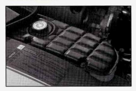
The coolant surge tank is in the engine compartment behind the headlamp.
