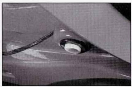
Tilt the driver's seat forward and press the storage compartment release button, or use the manual release cable if battery power has been lost. Lift the storage compartment lid (C). (After pressing the release button, the driver and passenger door glass should retract to the full-down position, if they have not already been lowered.)
