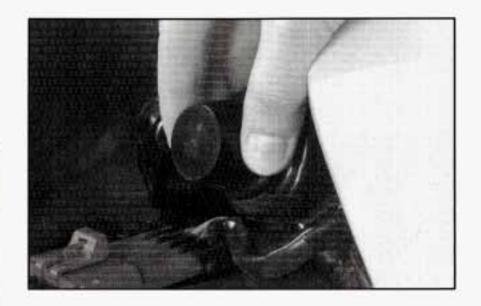
You can also open the headlamps manually by turning the adjuster to the left.
