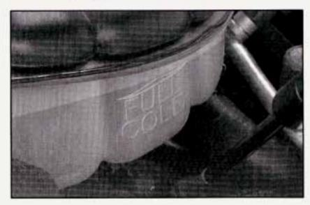
The coolant level should be at or above the FULL COLD mark.
