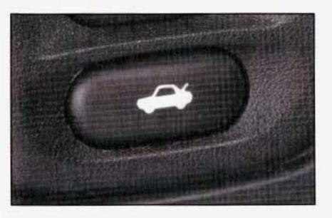
To use the remote hatch/trunk lid release on automatic transmission vehicles, your vehicle must be in PARK (P) or NUETRAL (N). For manual transmissions, set the parking brake. See "Parking Brake" in the Index.
