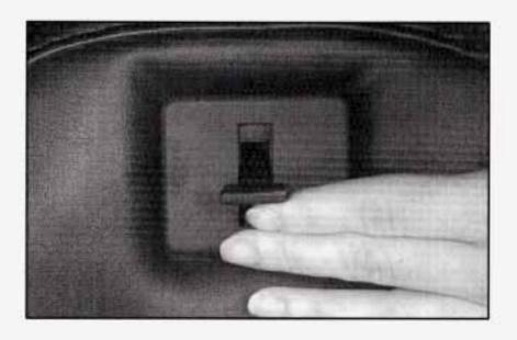
Both seatbacks fold forward to give you access to the rear area. To fold a seatback forward, lift this latch and pull the seatback forward. The seatback will lock down in this position. To unlock, lift up on the latch and push the seatback rearward. When you return the seatback to its original position, make sure the seatback is locked.
