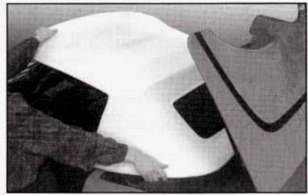
Push forward on the front edge (A) of the convertible top to allow the rear edge (B) of the convertible top to be rotated to its full-down position.
