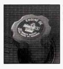
The engine oil fill cap is on top of the right valve rocker arm cover.
