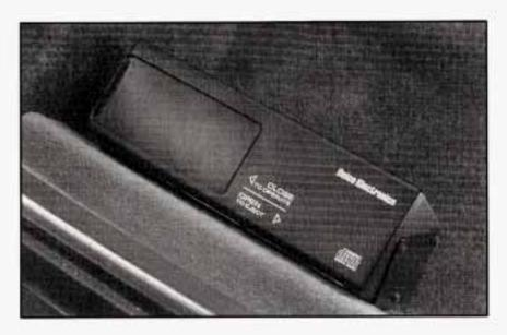
Your vehicle may be equipped with a trunk mounted CD changer. It is located in the rear center storage compartment. See "Rear Storage" in the Index for more information.
