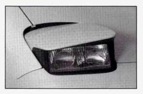
The headlamp doors are designed to open when you turn the headlamps on, and close when you turn the headlamps and parking lamps off. If you turn the headlamps on, then turn the headlamp switch back to the parking lamps setting, the headlamp doors will stay open. You can open the doors manually using the knob next to the headlamp assembly. Turn the knob to the left until the doors are open.
