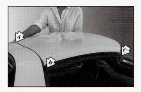
Position the rear edge of the roof panel to the weatherstrip on the back of the roof opening (A).
