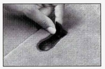
To access the center storage compartment, pull up on the two latches to release the carpet lid.
