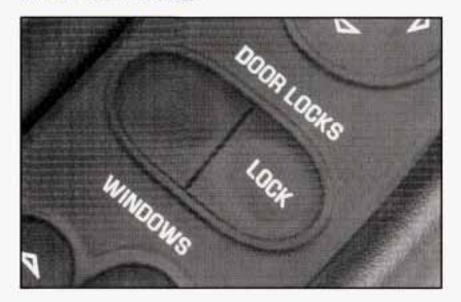
Press the power door unlock/lock switch on either door to lock or unlock both doors at once.
