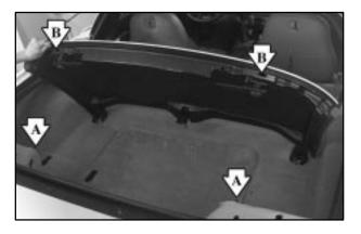
3. There are two spring-loaded storage pins on the rear wall of the storage compartment (A). These storage pins go into the slots on each side of the roof panel (B).
