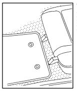
To remove the floor mats, pull up on the rear of the mat to disconnect from the locator hooks.
