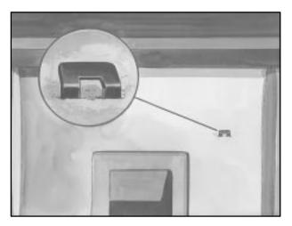
If your vehicle is a convertible or has a removable roof, don't use a child restraint with a top strap because the strap can't be anchored properly. You shouldn't use this type of child restraint without anchoring the top strap.
