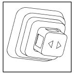
To operate the telescopic steering wheel, push the switch forward and the wheel will move away from you. Pull the switch rearward and the wheel will move toward you.
