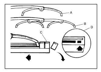
Slide the insert (D), notched end last, into the end with two blade claws (A). Slide the insert all the way through the blade claws at the opposite end (B). Plastic caps (C) will be forced off as the insert is fully installed.
