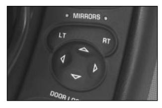
The electric mirror control is on the driver's door. It controls the driver's and passenger's mirrors. To adjust either mirror, press the LT (left) or RT (right) button to select the mirror, then press the arrows to adjust the direction of the mirror. The selected mirror will stay on for 20 seconds after the last adjustment. An indicator light will come on above the mirror that you select.
