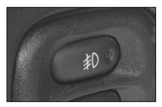
Use the fog lamps for better vision in foggy or misty conditions. Your parking lamps or low-beam headlamps must be on or the fog lamps won't work.
