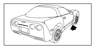
The front lifting point can be accessed from either the driver's or passenger's side of the vehicle, behind the front tires.
