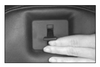
Both seatbacks fold forward to give you access to the rear area. To fold a seatback forward, lift this latch, which is located on top of the backside of the seat, and pull the seatback forward. The seatback will lock down in this position. To unlock, lift up on the latch and push the seatback rearward. When you return the seatback to its original position, make sure the seatback is locked.
