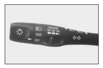
With cruise control, you can maintain a speed of about 25 mph (40 km/h) or more without keeping your foot on the accelerator. This can really help on long trips. Cruise control does not work at speeds below about 25 mph (40 km/h).
