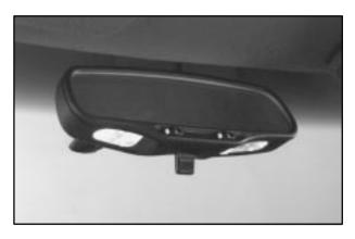
Your inside rearview mirror includes two reading lamps. The lamps will go on when a door is opened. When the doors are closed, each lamp can be turned on individually by pressing the switch (each lamp has its own switch).
