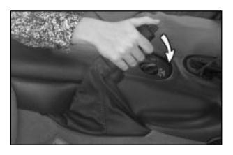
To release the parking brake, hold the brake pedal down. Then push the release button in as you move the parking brake lever all the way down.
