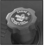
The engine oil fill cap is located on top of the valve cover on the passenger's side of the engine.
