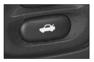
To use the hatch/trunk lid release on automatic transmission vehicles, your vehicle must be in PARK (P) or NEUTRAL (N). For manual transmissions, set the parking brake. See "Parking Brake" in the Index.
