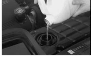
1. You can remove the coolant surge tank pressure cap when the cooling system, including the coolant surge tank pressure cap and upper radiator hose, is no longer hot. Turn the pressure cap slowly counterclockwise (left) about one-quarter turn and then stop.
