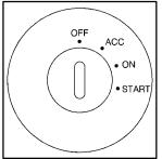
With the key in the ignition switch, you can turn the switch to four positions.
