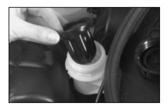
Fluid should be added if the fluid level is below the step on the inside of the reservoir. There are additional instructions on the reservoir cap. Put the rubber seal and cap back on.
