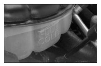
When the engine is cold, the coolant level should be at or above the FULL COLD mark. If it isn't, you may have a leak in the radiator hoses, heater hoses, radiator, water pump or somewhere else in the cooling system.
