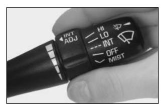
You can control the windshield wipers by moving the lever with the wiper symbol on it. This lever is located on the right-hand side of the steering column.
