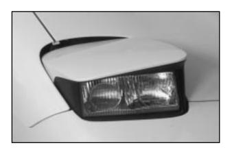
You can open the doors manually using the knob next to the headlamp assembly. Turn the knob counterclockwise until the doors are open. Turn the knob clockwise to close the doors manually.
