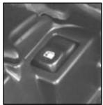
The fuel filler door release button is located inside of the center console storage compartment.
