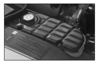
The coolant surge tank is located in the engine compartment behind the passenger's side headlamp.
