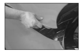
Then go to the side of the vehicle and pull up on the rear edge of the hood, near the windshield.
