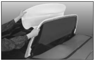
4. Lift upward on the front edge (A) of the convertible top off of the windshield frame. Then lift upward on the rear edge (B) of the convertible top to be vertical off the storage compartment lid (C). The front edge (A) and rear edge (B) should be straight up and down.
