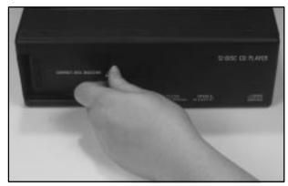
Close the door by sliding it all the way to the left. If the door is left partially open, the changer will not operate and an error will occur. When the door is closed, the changer will begin checking for discs in the magazine. This will continue for up to two minutes depending on the number of discs loaded.
