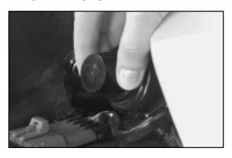
You can also open the headlamp doors manually by turning the adjuster counterclockwise.
