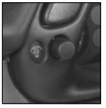
This knob controls the brightness of the instrument panel lights when the headlamps or parking lamps are on.
