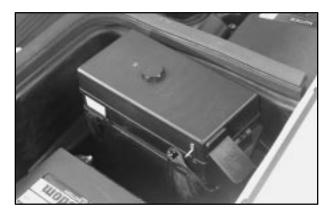
There is one fuse block in the engine compartment located on the passenger's side of the vehicle in front of the battery.
