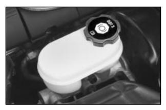
Your brake master cylinder reservoir is on the driver's side of the engine compartment. It is filled with DOT-3 brake fluid. See "Engine Compartment Overview" in the Index.
