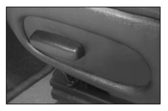
If your vehicle has this option, the control for the power seats will be located on the outboard side of each seat, near the base.
