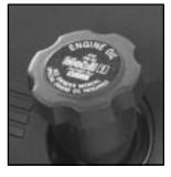
The engine oil fill cap is located in the engine compartment on top of the valve cover on the passenger's side of the vehicle. See "Engine Compartment Overview" in the Index for more information on location.
