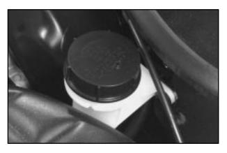
The clutch master cylinder reservoir is located at the rear of the engine compartment on the driver's side.
