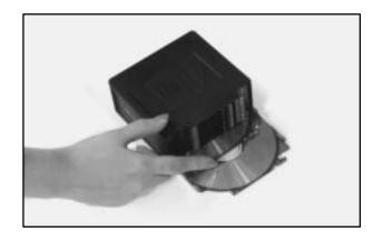
You must first load the magazine with discs before you can play a compact disc. Each of the 12 trays holds one disc. Press the button on the back of the magazine and pull gently on one of the trays. Load the trays from bottom to top, placing a disc on the tray label side down. If you load a disc label side up, the disc will not play and an error will occur. Gently push the tray back into the magazine slot. Repeat this procedure for loading up to 12 discs in the magazine.
