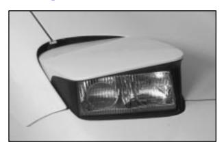
The headlamp doors are designed to open when you turn the headlamps on, and close when you turn the headlamps and parking lamps off. If you turn the headlamps on, then turn back to the parking lamps setting, the headlamp doors will stay open.
