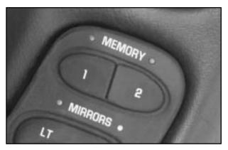
MEMORY can store and recall the settings for the driver's seat position, the outside rearview mirror positions, telescopic steering column (if equipped), radio presets, tone, volume, playback mode (AM/FM, tape or CD), last displayed station, compact disc position and tape direction and the last climate control setting.
