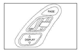
The HUD controls are located to the left of the steering wheel.
