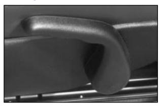
The lever for the reclining seatback is located on the outboard side of each seat, near the base.
