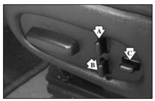
If your vehicle is equipped with a sport seat, there are three other controls that help you change the shape of the seat in addition to the power seat control. There are two lumbar supports for the middle (A) and lower (B) back. There's also a side bolster control (C) that adjusts the sides of the seat around you to give you more lateral support.
