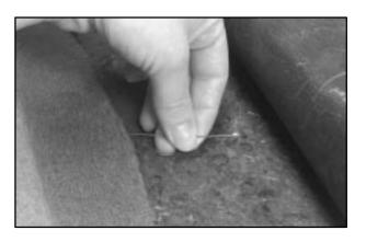
The cable is located underneath the carpeting behind the driver's and passenger's seats, in the center of the vehicle. When using the manual release, you must first open the doors to prevent damage to the seals. To access the cable, lift and pull back the carpeting. Then pull the cable to release the storage compartment lid if needed.
