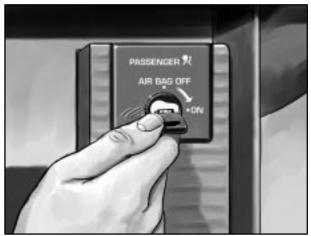
To turn the passenger's air bag on again, insert your ignition key into the switch, push in, and move the switch to the on position.
