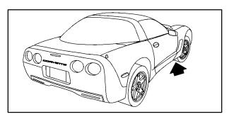
The front lifting point can be accessed from either the driver's or passenger's side of the vehicle, behind the front tires.
