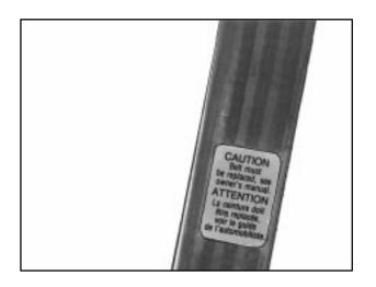
If you ever see a label on the driver's safety belt that says to replace the belt, be sure to do so. Then the new belt will be there to help protect you in a collision. You would see this label on the belt near the latch plate.
