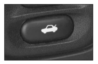
To use the hatch/trunk lid release on vehicles with an automatic transmission, your vehicle must be in PARK (P) or NEUTRAL (N). For manual transmissions, set the parking brake. See "Parking Brake" in the Index. Press the button with the trunk symbol on it, located at the left side of the steering column on the instrument panel, to release the hatch/trunk lid from inside your vehicle.
