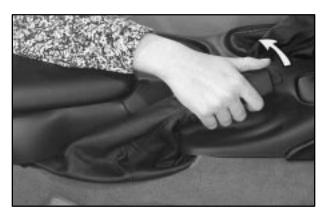
To set the parking brake, hold the brake pedal down. Pull the parking brake lever up. This sets your parking brake. If the ignition is on, the brake system warning light will come on.
