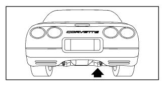
The rear lifting point can be accessed from the rear of the vehicle, on either the driver's or passenger's side.
