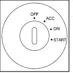
With the key in the ignition switch, you can turn it to four different positions.
