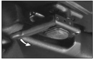
6. To unlock the front of the roof panel, pull down each of the front handles. Grasp the handles with your fingers and pull each toward you. Complete a 180° turn toward the center of the vehicle. Then push up on each of the handles.
