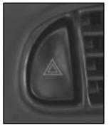
The hazard warning flasher button is located on the instrument panel above the audio system.
