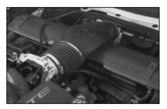
The engine air cleaner/filter is located at the center front of the engine compartment.
