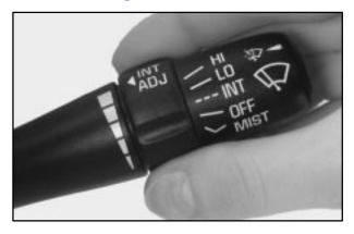
Use this lever located on the right side of the steering column to operate the windshield wipers.
