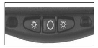
The mirror includes two map lamps and an automatic dimming function. There is also an interior console flood lamp located underneath the rearview mirror which remains on at all times.
