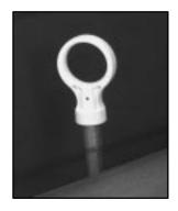
The engine oil dipstick handle is a yellow ring located near the coolant surge tank. See "Engine Compartment Overview" in the Index for more information on location.
