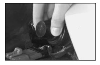
You can also open the headlamp doors manually by turning the adjuster counterclockwise.
