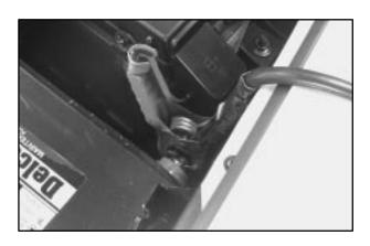
6. Connect the red positive (+) cable to the positive (+) terminal of the dead battery. Use a remote positive (+) terminal if the vehicle has one.
