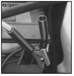
8. Now connect the black negative (-) cable to the negative (-) terminal of the good battery. Use a remote negative (-) terminal if the vehicle has one.
