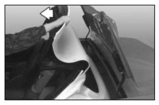
3. Pull the top up by firmly gripping the front edge (A) of the convertible top with your hand and applying a brisk, firm upward and forward motion to get the top in the full-up position.
