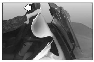
Pull the top up by firmly gripping the front edge (A)
