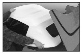
Push forward on the front edge (A) of the convertible top to allow the rear edge (B) of the convertible top to be moved to its full-down position.
