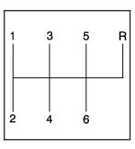
This is the shift pattern for the six-speed manual transmission.
