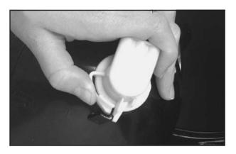
3. To remove the socket with the bulb, squeeze the tab while you turn the socket counterclockwise.
