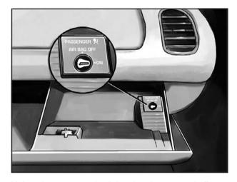
Unless the passenger's air bag has been turned off, *never* put a rear-facing child restraint in this vehicle.
