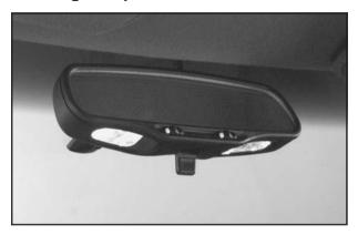
Your inside rearview mirror includes two reading lamps. The lamps will go on when a door is opened. When the doors are closed, each lamp can be turned on individually by pressing the switch for that lamp.
