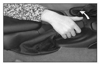
To set the parking brake, hold the brake pedal down. Pull the parking brake lever up. If the ignition is on, the brake system warning light will come on.
