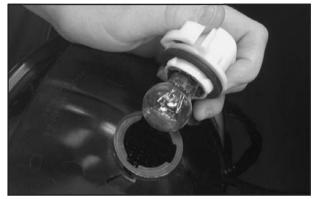
4. Remove the bulb from the socket.
