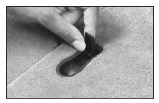
To access a storage compartment, pull up on the latch to release the lid. Remove the storage compartment lid. When replacing a storage compartment lid, make sure the latch is in the correct location so the latch locks securely into place.
