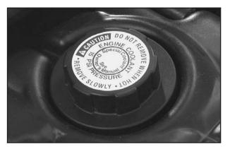
5. Then replace the pressure cap. Be sure the pressure cap is hand-tight and fully seated.
