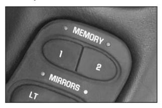
If your vehicle has this feature, MEMORY can store and recall the settings for the driver's seat position, the outside rearview mirror positions, telescopic steering column (if equipped), radio presets, tone, volume, playback mode (AM/FM, tape or CD), last displayed station, compact disc position and tape direction and the last climate control setting.
