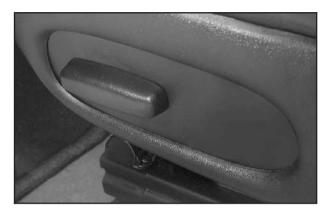
If your vehicle has this feature, the control for the power seats will be located on the outboard side of each seat, near the base.
