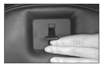
Both seatbacks fold forward to give you access to the rear area. To fold a seatback forward, lift this latch, which is located on top of the backside of the seat, and pull the seatback forward. The seatback will lock down in this position.
