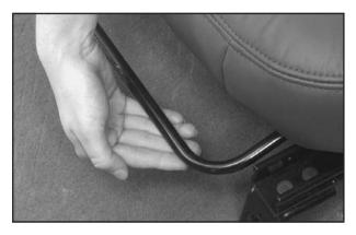
To move a manual seat, pull up on the lever located in front of the seat to unlock it. Slide the seat to where you want it and release the lever. Then try to move the seat with your body to make sure the seat is locked into place.
