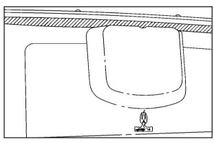
Notice: Using the emergency trunk release handle as a tie-down or anchor point when securing items in the trunk may damage it. Use the emergency trunk release handle only to help you open the trunk lid.
