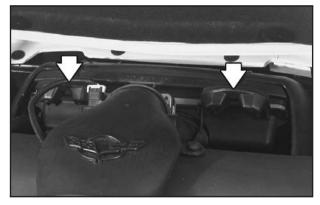
Pull up on the clips on each side to release the assembly.
