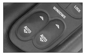
Both driver's and passenger's window switches have the express-down feature. Tap AUTO and immediately release. The window will lower completely. To stop the express-down feature from lowering the window completely, simply tap the switch again. You can also open the window any amount by pressing and releasing the switch.
