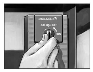
To turn off the passenger's air bag, insert your ignition key into the switch, push in, and move the switch to the off position.
