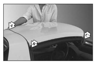
5. Position the rear edge of the roof panel to the weatherstrip on the back of the roof opening (A). Then align the pins at the rear of the roof panel weatherstrip with the receiving cup in the body weatherstrip (B). Gently lower the front edge of the roof panel to the front of the body opening (C).
