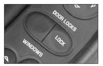
Press the power door switch on either door to unlock or lock both doors at once.
