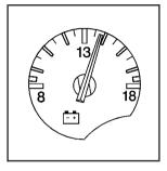
When the key is in ON with the engine not running, the voltmeter shows the voltage output of your battery. When the engine is running, it shows the voltage output of the charging system.
