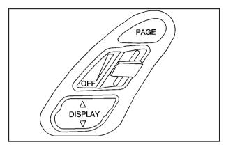
The HUD controls are located to the left of the steering wheel.
