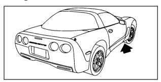
The front lifting point can be accessed for either the driver's or passenger's side of the vehicle, behind the front tires.
