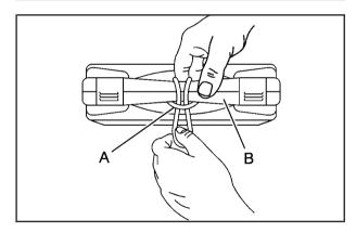
Loop the elastic cord (A) around the handle of the tire inflator kit.
