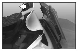
Tilt the driver's seat forward and press the storage compartment release button, or use the manual release cable if battery power has been lost. Lift the storage compartment lid (C). After pressing the release button, the driver and passenger door glass should retract to the full-down position, if they have not already been lowered.
