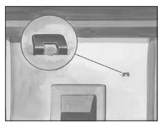
If your vehicle is a Z06, an anchor bracket for a top strap is located behind the passengers's seat in the cargo area. Anchor the top strap to the bracket.
