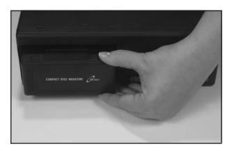
Once you have loaded the CDs in the magazine, slide open the door of the CD changer. Push the magazine into the changer in the direction of the arrow marked on top of the magazine.
