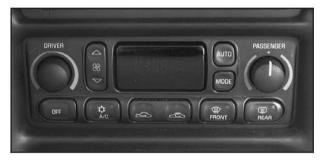
When your vehicle is first started, the display will show the driver's temperature setting, the fan speed and the air delivery for about five seconds; then it will show the outside temperature.
