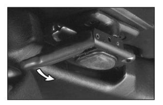
Unlock the front of the convertible top by lowering the latch handles and turning them inward. Push the latch handles back to the up position.
