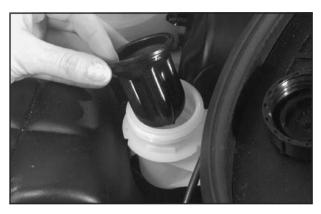
Fluid should be added if the fluid level is below the step on the inside of the reservoir. There are additional instructions on the reservoir cap. Put the rubber seal and cap back on. See *Engine Compartment Overview on page 5-12* for more information on location.
