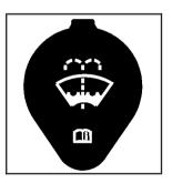
Open the cap with the washer symbol on it.
