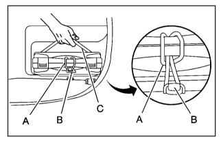
Remove the elastic cord (A) from around the retaining hook (B) and slide the kit out from under the elastic band (C) that is secured to the floor of the hatch/trunk area. Unwrap the elastic cord (A) from around the handle of the tire inflator kit. Open the tire inflator kit case by lifting up the two tabs located on either side of the kit handle. To Stow the Tire Inflator Kit:
