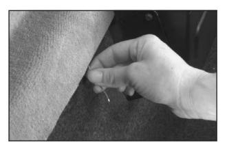
Pull the cable straight down to release the trunk lid. If your vehicle is equipped with a convertible top and trunk release handle and you have lost battery power, use the trunk release handle to open the trunk.
