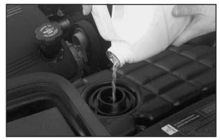
Then fill the coolant surge tank with the proper mixture, to the FULL COLD mark on the coolant surge tank.
