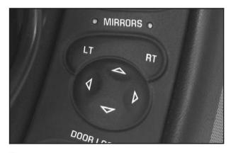
The power mirror control is on the driver's door. It controls the driver's and passenger's mirrors.
