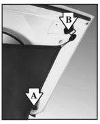
Hook the elastic loops on the front corners (A) of the shade to the T-nuts located on the front corners of the rear batch frame.
