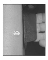
Pull the handle located inside the vehicle below the instrument panel on the driver's side.
