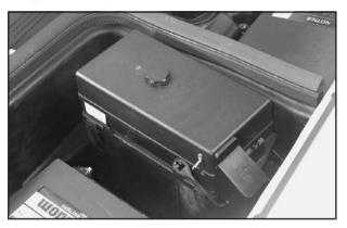
There is one fuse block in the engine compartment located on the passenger's side of the vehicle in front of the battery.
