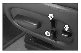
If your vehicle has this feature, there are three other controls that help you change the shape of the seat in addition to the power seat control. There are two lumbar supports for the middle (A) and lower (B) back. There is also a side bolster control (C) that adjusts the sides of the seat around you to give you more lateral support.
