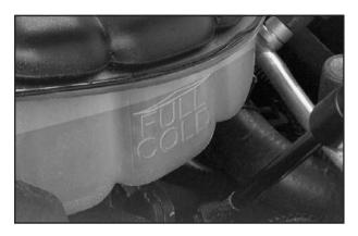
The coolant level should be at or above the FULL COLD mark. If it is not, you may have a leak at the pressure cap or in the radiator hoses, heater hoses, radiator, water pump or somewhere else in the cooling system.
