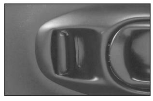
To lock the door from the inside, move the lever located on the door forward. To unlock it, move the lever on the door rearward.
