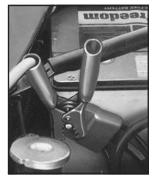
7. Do not let the other end touch metal. Connect it to the positive (+) terminal of the good battery. Use a remote positive (+) terminal if the vehicle has one.
