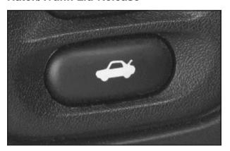
To use the hatch/trunk lid release on vehicles with an automatic transmission, your vehicle must be in PARK (P) or NEUTRAL (N). For manual transmissions, set the parking brake. See *Parking Brake on page 2-31*.
