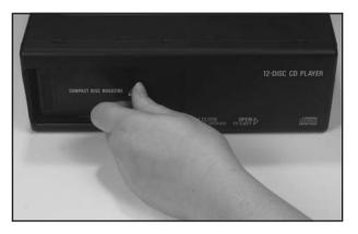
Close the door by sliding it all the way to the left. If the door is left partially open, the changer will not operate and an error will occur. When the door is closed, the changer will begin checking for CDs in the magazine. This will continue for up to two minutes depending on the number of CDs loaded.
