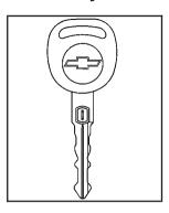
Your vehicle is equipped with the PASS-Key® (Personalized Automotive Security System) theft-deterrent system. PASS-Key® is a passive theft-deterrent system. It works when you insert or remove the key from the ignition.
