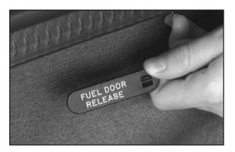
If your fuel filler door release will not operate, there is a manual release tab. The tab is located against the upper trim on the driver's side in the rear compartment. Pull the tab to manually release the fuel filler door.
