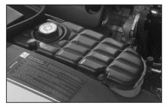
The coolant surge tank is located in the engine compartment behind the passenger's side headlamp. See *Engine Compartment Overview on page 5-12* for more information on location.
