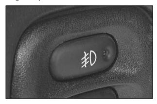
Your vehicle may have this feature. Use the fog lamps for better vision in foggy or misty conditions. Your parking lamps or low-beam headlamps must be on or the fog lamps will not work.
