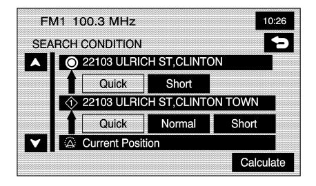
The search condition screen allows you to view your current destination and also change the planning methods between each destination. Each distance between waypoints and final destination can have an individual setting. Use the up/down arrows to scroll through your routes. Use the available route preference options to change your planning method. After selecting the new planning methods, touch Calculate to plan the route.
