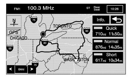
The system will calculate up to three different versions of your current route in three different colors: Quick, Normal, and Short. The routes are shown with distance to destination and estimated travel time. Touch the button corresponding to the route you want to choose.
