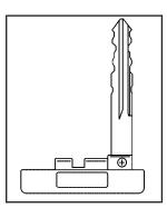
There is a key, located inside the keyless access transmitter, that works the glove box and can open the hatch/trunk lid if vehicle power is lost. See Hatch/Trunk on page 83 for more information.
