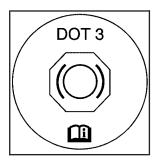
Your brake master cylinder reservoir is filled with DOT-3 brake fluid. See Engine Compartment Overview on page 328 for the location of the reservoir.
