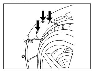
Access the high-beam or front parking/turn signal bulbs by removing the access panel. To do this, remove the three outer fasteners and move the cover back. Remove the outer cover to expose the high-beam headlamp bulb socket once the access cover has been removed.
