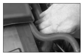
4. With the coolant surge tank pressure cap off, start the engine and let it run until you can feel the upper radiator hose getting hot. Watch out for the engine cooling fan.
