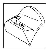
Insert the roof panel so that the outside front edges line up between the receiver covers. Push forward on the roof panel until it stops.
