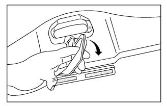
The convertible top front latch, located above the inside rearview mirror, must be unlocked. Pull the convertible top front latch down and turn it clockwise to unlock it.
