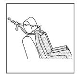
If the position you are using has a fixed head restraint and you are using a dual tether, route the tether around the head restraint.
