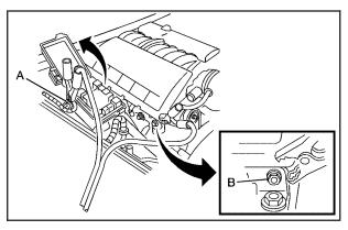
Your vehicle has a remote positive (+) terminal (A) and a remote negative (-) terminal (B), as shown in the illustration, which should be used to jump start your vehicle.
