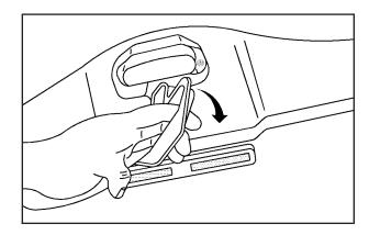
Release the convertible top front latch, located above the inside rearview mirror, by pulling and turning it clockwise toward the driver's door. Push upward on the front edge. The windows will automatically lower.
