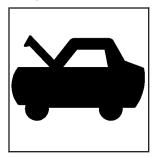
Pull the hood release lever with this symbol on it. It is located inside the vehicle below the instrument panel on the driver's side.
