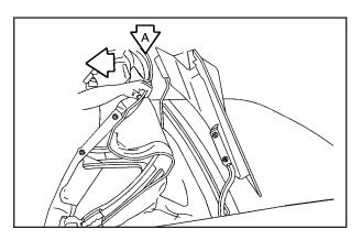
Pull the convertible top up by firmly gripping the front edge (A) near the center and applying a brisk upward and forward motion to get the top in the full-up position.
