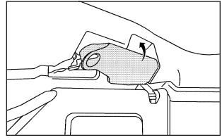
**Driver's Side Front Roof Panel Release Latch**
