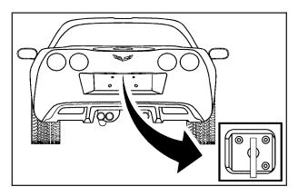
If your vehicle has lost battery power, open the hatch/trunk using the vehicle key located inside the keyless access transmitter. See *Keys on page 71* for more information. The key lock cylinder is located on the rear of the hatch/trunk lid above the license plate. Turn the vehicle key clockwise in the lock.
