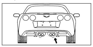
The rear lifting points can be accessed from the rear of the vehicle, on either the driver's or passenger's side.
