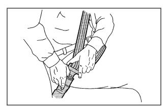
To unlatch the belt, push the button on the buckle. The belt should go back out of the way.
