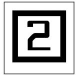
When using the Manual Paddle Shift Feature while in the SPORT MODE (S), the current gear will be displayed in the Driver Information (DIC), or the Head-Up Display (HUD), if the vehicle has either of these features.
