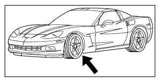
The front lifting points can be accessed from either side of your vehicle, behind the front tires.
