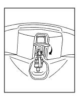
6. Turn the front release handles inward so that they latch to the closed position.
