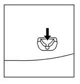
Gently place the roof panel down so that the back pins on the roof panel drop into the receivers in the back of the storage area.
