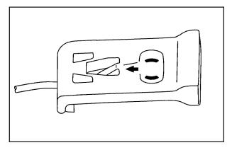
From outside the vehicle, use the key in the cylinder above the license plate to open the hatch the use the door release tab located on the carpet inside the trunk on the driver's side of the vehicle. Pull the tab to unlock and unlatch the driver's door. See *Keys on page 71* for information on opening the trunk during a loss of power.
