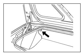
Pull the divider up and snap it onto the snaps on both sides of the trunk.
