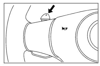
While in the SPORT MODE (S) mode, push the paddle above the steering wheel spokes to up-shift to the next gear, or pull on the paddle behind the steering wheel spokes to down-shift to the next gear.
