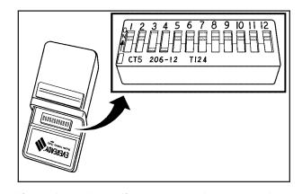
If you do not know if your garage door opener is a fixed code or rolling code device, open your garage door opener's remote control battery cover. Your garage door opener is a fixed code device if there is a panel of switches. If not, your garage door opener is a rolling code device.
