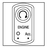
Your vehicle has an electronic keyless ignition with a pushbutton start.
