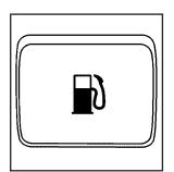
The fuel door release button is located on the instrument panel to the left of the steering wheel. Push the button to release the fuel door.
