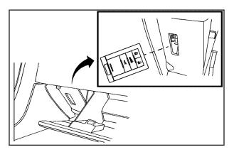
If moving the transmitter to different locations within the vehicle does not help, place the transmitter in the glove box transmitter pocket with the buttons facing to the right and then press the START button.
