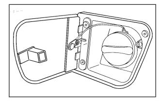
The tethered fuel cap is located behind a hinged fuel door on the driver's side of the vehicle.
