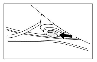
6. Tilt the driver's seatback forward and press the tonneau cover release button located on the underside of the tonneau cover (C) behind the driver's seat. Then raise the tonneau cover (C). If the tonneau cover does not release and three chimes are heard, check to make sure the trunk lid is closed. Also, the cover will not release if the vehicle alarm is armed. After pressing the release button, the driver's and passenger's door glass should retract to the full-down position.
