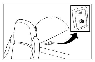
The top tether anchor is located behind the passenger seat.
