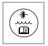
The hydraulic clutch fluid reservoir cap has this symbol on it. See *Engine Compartment Overview on page 328* for reservoir location.
