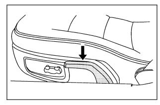
To adjust the seatback, lean slightly forward to lift your weight off the seatback. Pull completely up on the lever until it stops, and lean back to position the seatback to where you want it. Release the lever to lock the seatback into place.
