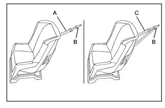
A top tether (A, C) anchors the top of the child restraint to the vehicle. A top tether anchor is built into the vehicle.
