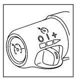
(Off): Slide the switch to this position to turn the system off.
