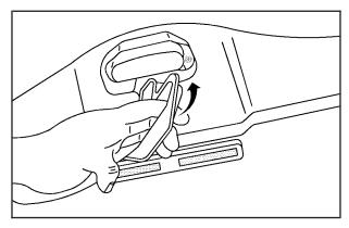
11. Pull the top front latch handle down and turn it counterclockwise to lock the convertible top.
