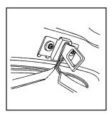
Push the loop to the top of the striker (base plate).
