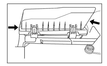
If you are cleaning your vehicle with the hood open, take care not to spray water directly into either end of the air cleaner/filter housing, as shown in the illustration, as this could damage your vehicle's engine.
