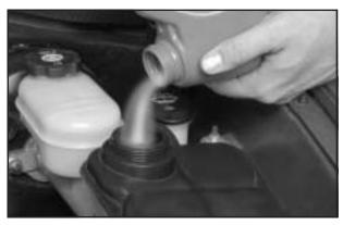
Fill the coolant surge tank with the proper mixture until the level inside stabilizes at the FULL COLD mark on the front of the surge tank.
