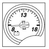
The voltmeter shows the voltage output of your battery. When the engine is running, it shows the voltage output of the charging system.
