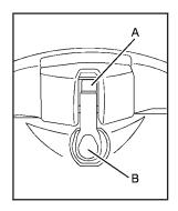
7. To unlock the rear of the roof panel's rear release latch, press the back of the release handle (B). Then press the button on the front of the release handle, (A) with your thumb.
