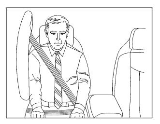
If your vehicle has a side impact airbag for the right front passenger, it is in the side of the passenger's seatback closest to the door.
