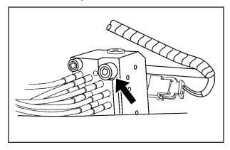
2. Locate the pressure release bolt on the front side of the hydraulic pump.
