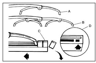
Slide the insert (D), notched end last, into the end with the two blade claws (A). Slide the insert all the way through the blade claws at the opposite end (B). Plastic caps (C) will be forced off as the insert is fully installed.
