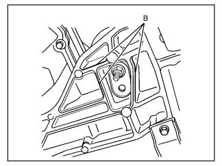
Lift the vehicle with the jack, making sure the jack spans at least two of the crossmember ribs (B).
