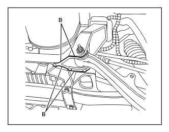
Lift the vehicle with the jack, making sure the jack spans at least two of the crossmember ribs (B).
