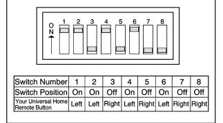
**Example of Eight Dip Switches with Two Positions**
