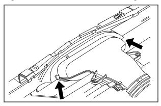
If you are cleaning your vehicle with the hood open, take care not to spray water directly near the filter opening of the air cleaner, as shown in the illustration, as this could damage your vehicle's engine.
