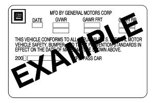
A vehicle specific Certification label is attached to the rear edge of the driver's door. It tells you the gross weight capacity of your vehicle, called the Gross Vehicle Weight Rating (GVWR). The GVWR includes the weight of the vehicle, all occupants, fuel and cargo. Never exceed the GVWR for your vehicle, or the Gross Axle Weight Rating (GAWR) for either the front or rear axle.
