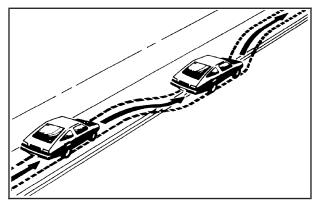
If the level of the shoulder is only slightly below the pavement, recovery should be fairly easy. Ease off the accelerator and then, if there is nothing in the way, steer so that your vehicle straddles the edge of the pavement. You can turn the steering wheel up to one-quarter turn until the right front tire contacts the pavement edge. Then turn the steering wheel to go straight down the roadway.
