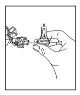
Remove the headlamp bulb by releasing the outer tabs from the socket.
