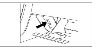
If moving the transmitter to different locations within the vehicle does not help, place the transmitter in the glove box transmitter pocket with the buttons facing to the right and then press the START button.
