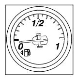
The fuel gage shows how much fuel the vehicle has left while the engine is on.
