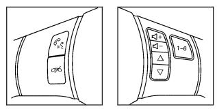
For vehicles with steering wheel controls, some audio controls can be adjusted at the steering wheel.
