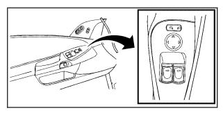
Controls for the outside power mirrors are located on the driver door.
