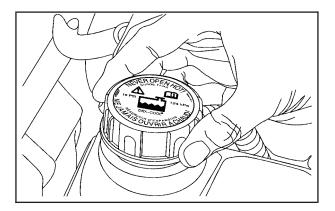
1. When the cooling system, including the coolant surge tank pressure cap and upper radiator hose, is no longer hot, remove the pressure cap.
