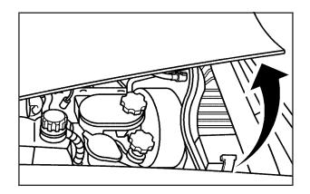
2. Go to the side of the vehicle and pull up on the rear edge of the hood, near the windshield.
