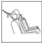
If the position you are using has a fixed headrest or head restraint and you are using a dual tether, route the tether around the headrest or head restraint.
