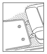
To reinstall the floor mats, position the openings in the floor mat over the locator pins and push it down into place.
