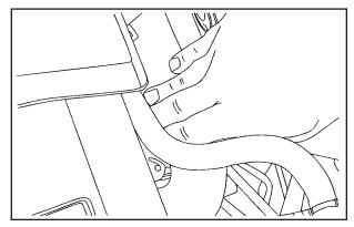
4. With the coolant surge tank pressure cap off, start the engine and let it run until you can feel the upper radiator hose getting hot. Any time during this procedure, watch out for the engine cooling fan.
