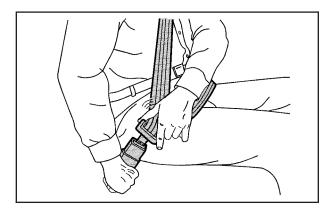
3. Push the latch plate into the buckle until it clicks. Pull up on the latch plate to make sure it is secure. If the belt is not long enough, see *Safety Belt Extender on page 1-25*.
