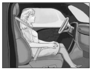
If a person of adult-size is sitting in the right front passenger seat, but the off indicator is lit, it could be because that person is not sitting properly in the seat. If this happens, use the following steps to allow the system to detect that person and enable the right front passenger frontal airbag and seat-mounted side impact airbag (if equipped):
