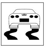
The Traction Control System (TCS) Warning light comes on briefly while starting the engine.
