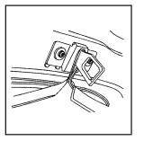
4. Push the loop to the top of the striker (base plate).
