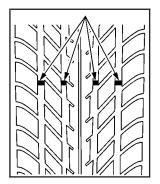
One way to tell when it is time for new tires is to check the treadwear indicators, which will appear when your tires have only 1/16 inch (1.6 mm) or less of tread remaining. You need a new tire if any of the following statements are true:
