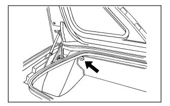
Pull the divider up and snap it onto the snaps on both sides of the trunk.
