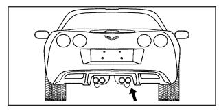
The rear lifting points can be accessed from the rear of the vehicle, on either the driver's or passenger's side.
