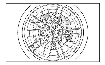
A rotor protector should always be installed before any wheel removal. The protector can be installed by feeding it through the wheel spokes and slipping it over the outer edge of the rotor. Leave the protector in place, over the rotor edge, until the wheel is re-installed. Rotor protectors are available through your dealer/retailer.
