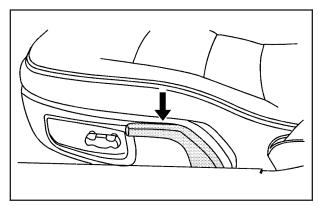
To adjust the seatback, lean slightly forward to lift your weight off the seatback. Pull completely up on the lever until it stops, and lean back to position the seatback to where you want it. Release the lever to lock the seatback into place.
