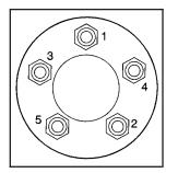
Tighten the wheel lug nuts firmly in a crisscross sequence as shown.
