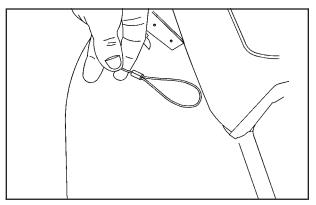
1. Open the tonneau cover by pulling the emergency release cable.
