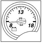
The voltmeter shows the voltage output of the battery. It shows the voltage output of the charging system while the engine is running.
