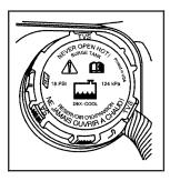
The engine coolant surge tank is located toward the rear of the engine compartment on the driver side of the vehicle. See Engine Compartment Overview on page 5-14 for more information on location. When the engine is cold, the coolant level should be at the FULL COLD mark on the coolant surge tank.
