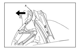
6. Pull the convertible top up by firmly gripping the front edge (A) near the center and applying a brisk upward and forward motion to get the top in the full-up position.
