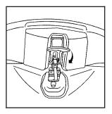
6. Turn the front release handles inward so that they latch to the closed position.
