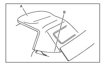
Push forward on the front edge (A) of the convertible top to allow the rear edge (B) of the convertible top to be moved to its full-down position.
