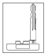
The key, located inside the keyless access transmitter, can be used to lock and unlock the glove box and to open the hatch/trunk lid if power to the vehicle is lost. See *Hatch on page 2-14* for more information.
