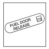
There is also a manual fuel door release tab. It is located against the upper trim in the rear compartment on the driver side of the vehicle. Pull the tab to release the fuel door.
