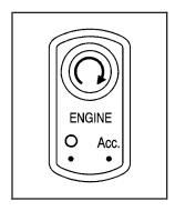
The vehicle has an electronic keyless ignition with a pushbutton start.
