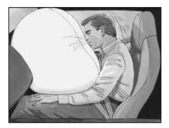
The right front passenger frontal airbag is in the instrument panel on the passenger's side.
