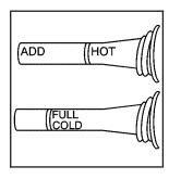
When the engine compartment is hot, the level should be at the HOT mark. When the engine compartment is cool, the level should be at the FULL COLD mark.
