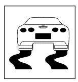
The Active Handling System light comes on briefly as the engine is started. If the light does not, have the vehicle serviced by your dealer/retailer. If the system is working normally the light goes off. If the light stays on or comes on while driving, a chime sounds and a SERVICE ACTIVE HANDLING SYSTEM message appears on the DIC and the vehicle need service.
