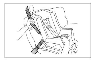
6. To tighten the belt, push down on the child restraint, pull the shoulder portion of the belt to tighten the lap portion of the belt and feed the shoulder belt back into the retractor. When installing a forward-facing child restraint, you may find it helpful to use your knee to push down on the child restraint as you tighten the belt.
