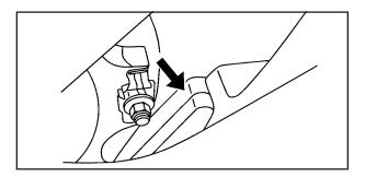
The ZR1 also has an electronic brake pad wear sensor system. When pads are worn, the CHANGE BRAKE PADS message displays in the Driver Information Center. See *DIC Warnings and Messages on page 3-56.*
