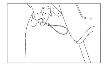
7. Pull the cable to release the tonneau cover.
