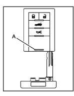
Press the button (A) near the bottom of the keyless access transmitter to remove the key. Never pull the key out without pressing the button. This vehicle has a keyless access system with pushbutton start. See *Ignition Positions on page 2-23* for information on starting the vehicle.
