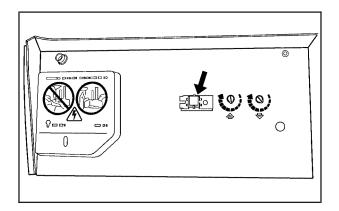
3. Locate in the garage, the garage door opener receiver (motor-head unit). Locate the "Learn" or "Smart" button. It can usually be found where the hanging antenna wire is attached to the motor-head unit and may be a colored button. Press this button. After pressing this button, complete the following steps in less than 30 seconds.
