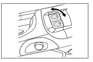
The power window switches are located on each door.
