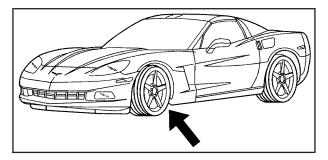
The front lifting points can be accessed from either side of your vehicle, behind the front tires.
