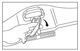
4. The convertible top front latch, located above the inside rearview mirror, must be unlocked. Pull the convertible top front latch down and turn it clockwise to unlock it.
