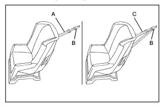
A top tether (A, C) anchors the top of the child restraint to the vehicle. A top tether anchor is built into the vehicle. The top tether attachment (B) on the child restraint connects to the top tether anchor in the vehicle in order to reduce the forward movement and rotation of the child restraint during driving or in a crash. Your child restraint may have a single tether (A) or a dual tether (C). Either will have a single attachment (B) to secure the top tether to the anchor.
