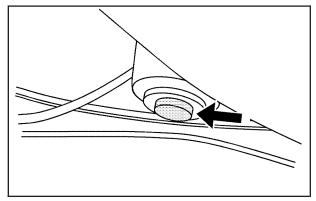
6. Tilt the driver's seatback forward and press the tonneau cover release button located on the underside of the tonneau cover (C) behind the driver's seat. Then raise the tonneau cover (C). If the tonneau cover does not release and three chimes are heard, check to make sure the trunk lid is closed. Also, the cover will not release if the vehicle alarm is armed.
