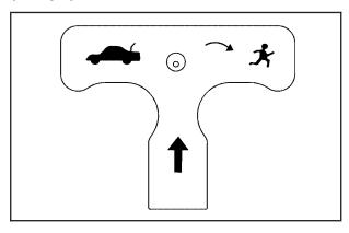
*Notice:* Do not use the emergency trunk release handle as a tie-down or anchor point when securing items in the trunk as it could damage the handle.
