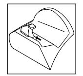
Insert the roof panel so that the outside front edges line up between the receiver covers. Push forward on the roof panel until it stops.
