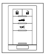
**(Lock):** Press once to lock the doors. When **i** is pressed twice, the lights flash and the horn sounds to confirm locking.
