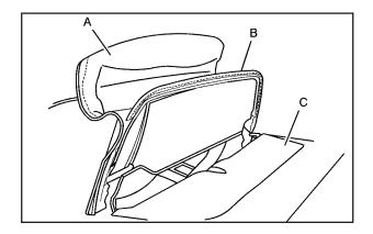
Lift upward on the front edge (A) of the convertible top off of the windshield frame. Then lift upward on the rear edge (B) of the convertible top so it is vertical to the tonneau cover (C). The front edge (A) and rear edge (B) should be straight up.
