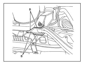
3. Lift the vehicle with the jack, making sure the jack spans at least two of the crossmember ribs (B).
