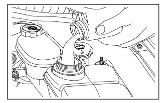
Fill the coolant surge tank with the proper DEX-COOL coolant mixture until the level inside stabilizes at the FULL COLD mark on the front of the surge tank.
