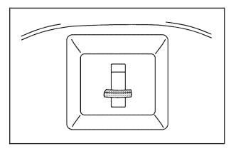
To fold a seatback forward, lift the latch located on top of the backside of the seat. The seatback locks when folded down. To return the seatback upright, lift up on the latch and push the seatback rearward. The seatback must be locked in place.
