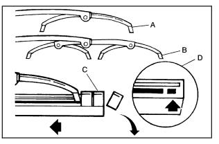
Slide the insert (D), notched end last, into the end with the two blade claws (A). Slide the insert all the way through the blade claws at the opposite end (B). The plastic caps (C) will be forced off as the insert is fully installed.
