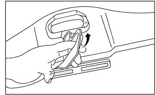
11. Pull the top front latch handle down and turn it counterclockwise to lock the convertible top.
