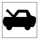
1. Pull the hood release lever with this symbol on it. It is located inside the vehicle below the instrument panel on the driver side.
