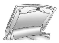
3. Grasp the loop at the rear center of the shade and wrap it around the striker assembly.
