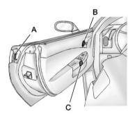
When you have the transmitter with you, you may also unlock and open the door by squeezing the door handle sensor (A).
