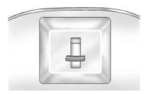
To fold a seatback forward, lift the latch on top of the backside of the seat. The seatback locks when folded down.
