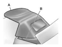
Push forward on the front edge (A) of the convertible top to allow the rear edge (B) of the convertible top to be moved to its full-down position.
