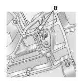
Lift the vehicle with the jack, making sure the jack spans at least two of the crossmember ribs (B).
