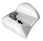
Insert the roof panel so that the outside front edges line up between the receiver covers. Push forward on the roof panel until it stops.
