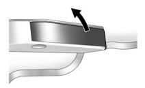
From inside the vehicle, use the door release handle located on the floor next to each seat. Pull the handle up to unlock and unlatch the door.
