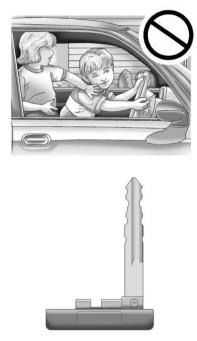
The key located inside the RKE transmitter can be used to lock and unlock the glove box and to open
