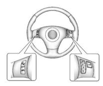
For vehicles with steering wheel controls, some audio controls can be adjusted at the steering wheel.
