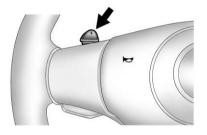
To operate the Manual Paddle Shift system, the automatic transmission shifter must be in S (Sport Mode). The system is activated by pushing the paddle, above the steering wheel spokes, to manually up-shift to the next gear, or pulling on the paddle, behind the steering wheel spokes to manually down-shift. The current gear will be displayed in the Driver Information (DIC), or the Head-Up Display (HUD), if the vehicle has either of these features.
