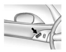
On vehicles with the memory feature, the controls on the driver door are used to program and recall memory settings for the driver seat, outside mirrors, and the telescopic steering column, if equipped. The numbers on the back of the remote keyless entry (RKE) transmitters correspond to the numbers on the memory buttons.
