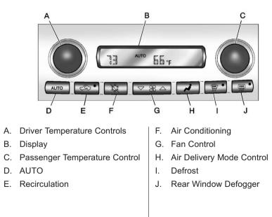
When the vehicle is first started, the display shows the driver's temperature setting, the outside temperature, the fan speed, and the air delivery, for about 10 seconds.
