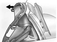
Pull the convertible top up by firmly gripping the front edge (A) near the center and applying a brisk upward and forward motion to get the top in the full-up position.
