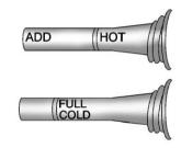
When the engine compartment is hot, the level should be at the HOT mark. When the engine compartment is cool, the level should be at the FULL COLD mark.
