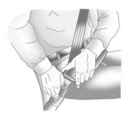
To unlatch the belt, push the button on the buckle. The belt should return to its stowed position.
