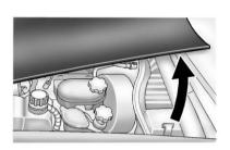
2. Go to the side of the vehicle and pull up on the rear edge of the hood, near the windshield.
