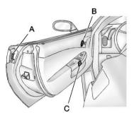
When you have the transmitter with you, you may also unlock and open the door by squeezing the door handle sensor (A). You do not have to press the unlock button on the transmitter. You will be able to open the door when you press the door handle sensor and the vehicle recognizes your keyless access transmitter. When the passenger door is opened first, the driver door will also unlock.
