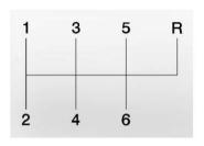
This is the shift pattern for the six-speed manual transmission.
