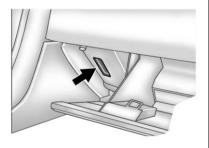
If moving the transmitter to different locations within the vehicle does not help, place the transmitter in the glove box transmitter pocket with the buttons facing to the right and then press the START button.  The vehicle's battery voltage is low. The battery voltage must be above 10 volts for the RKE transmitter to be detected properly.
