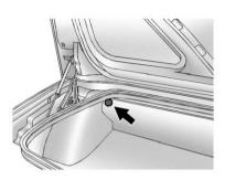
Pull the divider up and snap it onto the snaps on both sides of the trunk.
