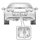
Press the hatch/trunk release button located on the rear of the hatch/ trunk lid above the license plate, as long as you have your transmitter with you. If your vehicle has lost battery power, open the hatch/trunk using the vehicle key. See *Keys on page 2-2* for more information. The key lock cylinder is located on the rear of the hatch/trunk lid above the license plate. Turn the vehicle key clockwise in the lock.
