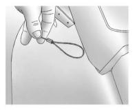
8. Pull the cable to release the tonneau cover.
