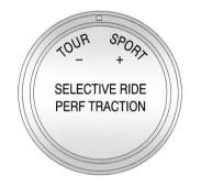
This knob is located on the center console. Turn it to select the suspension of your choice. The knob will return to the center position when released. The switch will illuminate the current suspension setting.
