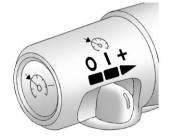
The vehicle has cruise control. O (Off): Turns the system off. I (On): Turns the system on.
