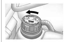
When the cooling system, including the coolant surge tank pressure cap and upper radiator hose, is no longer hot, remove the pressure cap.
