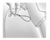
1. Open the tonneau cover by pulling the emergency release cable.
