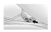
7. Tilt the driver seatback forward and press the tonneau cover release button located on the underside of the tonneau cover (C) behind the driver seat. Then raise the tonneau cover (C). If the tonneau cover does not release and three chimes are heard, check to make sure the trunk lid is closed. Also, the tonneau cover will not release if the vehicle alarm is armed. After pressing the release button, the driver and passenger door glass should retract to the full-down position.
