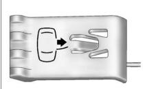
• From outside the vehicle, use the key in the cylinder above the license plate to open the hatch. Then, use the door release tab, located on the carpet inside the hatch on the driver side of the vehicle. Pull the tab to unlock and unlatch the driver door. See *Keys on page 2-2* for information on opening the hatch during a loss of power.
