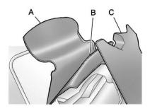
Lift the rear edge (B) of the convertible top to its full-up position by first raising the front edge (A).
