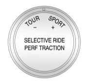
To select a mode while in Performance Traction Management, turn the knob located on the console.
