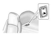
The top tether anchor is located under the cover behind the passenger seat. Securing a Child Restraint with a Top Tether
