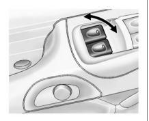
The power window switches are located on each door.
