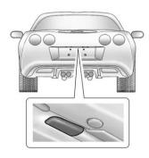
Push the hatch/trunk release button with the keyless entry transmitter within range. See Remote Keyless Entry (RKE) System on page 2-3.
