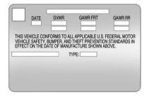
A vehicle-specific Certification label is attached to the rear edge of the driver door.
