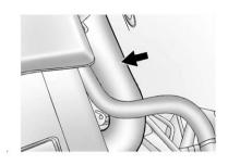
4. With the coolant surge tank pressure cap off, start the engine and let it run until the upper radiator hose can be felt getting hot. Any time during this procedure, watch out for the engine cooling fan.
