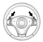
The Manual Paddle Shift system is activated from S (Sport Mode) by pushing the paddle, above the steering wheel spokes, to up-shift to the next gear, or pulling on the paddle, behind the steering wheel spokes, to down-shift to the next gear.
