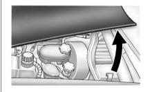
Go to the side of the vehicle and pull up on the rear edge of the hood, near the windshield.
