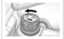
When the cooling system, including the coolant surge tank pressure cap and upper radiator hose, is no longer hot, remove the pressure cap.
