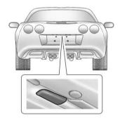
Push the hatch/trunk release button with the RKE transmitter within range. See Remote Keyless Entry (RKE) System on page 2-3.
