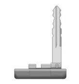
The key located inside the RKE transmitter can be used to lock and unlock the glove box and to open
