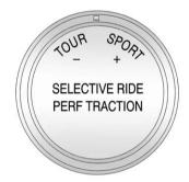
To select a mode while in Performance Traction Management, turn the knob located on the center console. The Performance Traction
