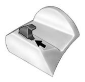
Insert the roof panel so that the outside front edges line up between the receiver covers.
