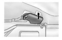
To unlock the release latches on the front of the roof panel, grasp each handle and pull it outward.
