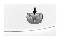
Gently place the roof panel down so that the back pins on the roof panel drop into the receivers in the back of the storage area.
