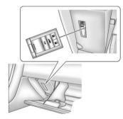
Place the new transmitter in the glove box transmitter pocket with the buttons facing the passenger side.
