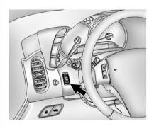
Push and hold ∨ on the convertible top switch. The convertible top will lower into the rear of the vehicle. A chime will sound when the convertible top has lowered completely. If the radio is on, the sound may be muted for a brief time due to a new audio system equalization being loaded.
