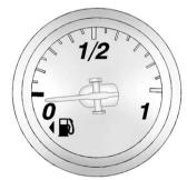
The fuel gauge shows how much fuel the vehicle has left while the engine is on.
