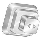
For vehicles with this feature, the telescopic steering column control is located on the right side of the steering column.
