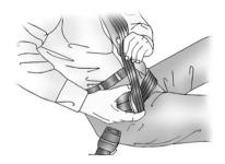
If the belt stops before it reaches the buckle, tilt the latch plate and keep pulling the safety belt until it can be buckled.
