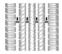
Treadwear indicators are one way to tell when it is time for new tires. Treadwear indicators appear when the tires have only 1.6 mm (1/16 in) or less of tread remaining. See *Tire Inspection on page 10-68* and *Tire Rotation on page 10-68* for more information.
