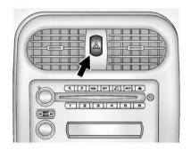
The hazard warning flashers warn others that you have a problem. The button is located near the center of the instrument panel.
