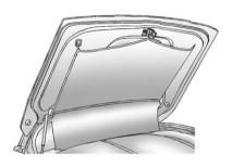
Grasp the loop at the rear center of the shade and wrap it around the striker assembly.
