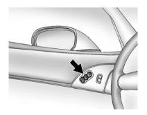
On vehicles with the memory feature, the controls on the driver door are used to program and recall memory settings for the driver seat, outside mirrors, and the telescopic steering column.
