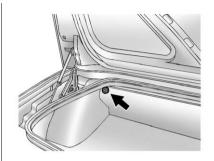
Pull the divider up and snap it onto place on both sides of the trunk.
