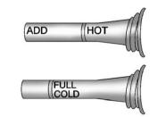
When the engine compartment is hot, the level should be at the HOT mark.
