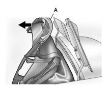
6. Pull the convertible top up by firmly gripping the front edge (A) near the center and applying a brisk upward and forward motion to get the top in the full-up position.
