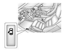
• From inside the vehicle, pull the door release handle.
