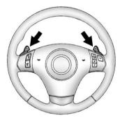
The Manual Paddle Shift system can be used in D (Drive) or S (Sport Mode). The system is activated by pushing the paddle, above the steering wheel spokes, to manually up-shift to the next gear, or pulling on the paddle, behind the steering wheel spokes to manually down-shift.
