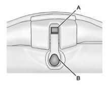
7. To unlock the rear of the roof panel's rear release latch, press the back of the release handle (B). Then press the button on the front of the release handle (A).
