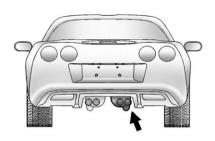
The rear lifting points can be accessed from the rear of the vehicle, on either the driver's or passenger's side.
