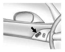
On vehicles with the memory feature, the controls on the driver door are used to program and recall memory settings for the driver seat, outside mirrors, and the telescopic steering column, if equipped.
