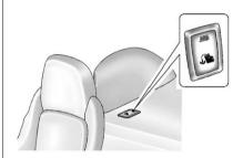
The top tether anchor is located under the cover behind the passenger seat.
