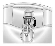
Turn the front release handles inward so that they latch to the closed position.
