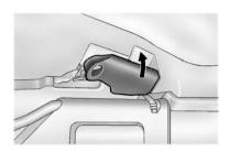
6. To unlock the release latches on the front of the roof panel, grasp each handle and pull it outward.
