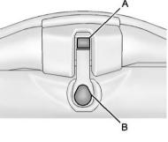
7. To unlock the rear of the roof panel's rear release latch, press the back of the release handle (B). Then press the button on the front of the release handle (A).
