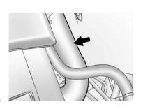
4. With the coolant surge tank pressure cap off, start the engine and let it run until the upper radiator hose can be felt getting hot. Any time during this procedure, watch out for the engine cooling fan.
