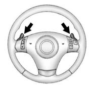
The Manual Paddle Shift system can be used in D (Drive) or S (Sport Mode). The system is activated by pushing the paddle, above the steering wheel spokes, to manually up-shift to the next gear, or pulling on the paddle, behind the steering wheel spokes to manually down-shift. The current gear will be displayed in the Driver Information (DIC), or the Head-Up Display (HUD), if the vehicle has either of these features.
