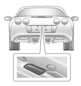
Press the hatch/trunk release touch pad with the keyless entry transmitter within range. See Remote Keyless Entry (RKE) System on page 2-2.
