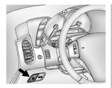
The fuel door release button is located on the instrument panel to the left of the steering wheel. Push the button to release the fuel door.
