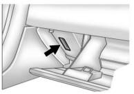
If moving the transmitter to different locations within the vehicle does not help, place the transmitter in the glove box transmitter pocket with the buttons facing to the right and then press the START button.
