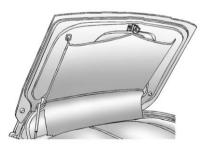
3. Grasp the loop at the rear center of the shade and wrap it around the striker assembly.
