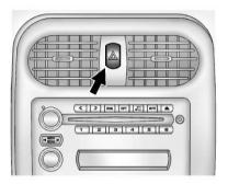
The hazard warning flashers warn others that you have a problem. The button is located near the center of the instrument panel.
