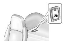
The top tether anchor is located under the cover behind the passenger seat. Securing a Child Restraint with a Top Tether
