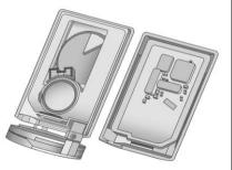
Separate the transmitter with a flat, thin object inserted into the slot on the side of the transmitter.
