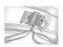
4. Push the loop to the top of the striker (base plate).
