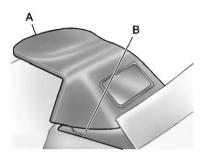
Push forward on the front edge (A) of the convertible top to allow the rear edge (B) of the convertible top to be moved to its full-down position.
