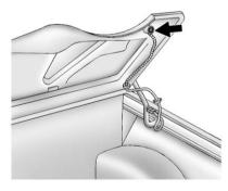
4. Tilt the driver seat forward and press the tonneau cover release button. After pressing the release button, the driver and passenger door glass will retract to the full-down position. If battery power has been lost, see Step 7 under "Lowering the Manual Convertible Top" in this section.
