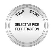
This knob is on the center console. Turn it to select the suspension of your choice. The knob will return to the center position when released. The switch will illuminate the current suspension setting.
