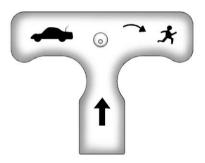
*Notice:* Do not use the emergency trunk release handle as a tie-down or anchor point when securing items in the trunk as it could damage the handle. The emergency trunk release handle is only intended to aid a person trapped in a latched trunk, enabling them to open the trunk from the inside.
