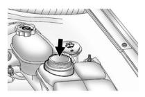
Fill the coolant surge tank with the proper DEX-COOL coolant mixture until the level inside stabilizes at the FULL COLD mark on the front of the surge tank.
