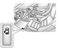
• From inside the vehicle, pull the door release handle.
