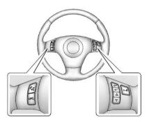
For vehicles with steering wheel controls, some audio controls can be adjusted at the steering wheel.
