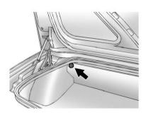
Pull the divider up and snap it onto place on both sides of the trunk.
