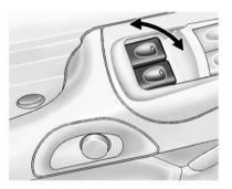
Pull up or press down on the front of the switch to raise or lower the window.
