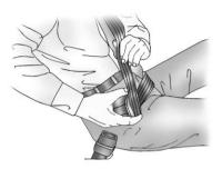
3. If the belt stops before it reaches the buckle, tilt the latch plate and keep pulling the safety belt until it can be buckled.
