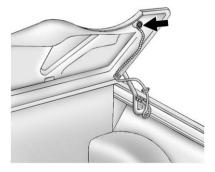
Tilt the driver seatback forward and press the tonneau cover release button located on the underside of the tonneau cover (C) behind the driver seat. After pressing the release button, the driver and passenger door glass will retract to the full-down position. Then raise the tonneau cover (C).
