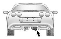
The rear lifting points can be accessed from the rear of the vehicle, on either the driver's or passenger's side.
