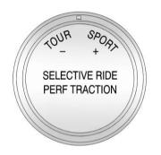
To select a mode while in Performance Traction Management, turn the knob on the center console.
