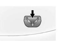
Gently place the roof panel down so that the back pins on the roof panel drop into the receivers in the back of the storage area.
