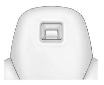
To fold a seatback forward, lift the latch on top of the backside of the seat. The seatback locks when folded down.
