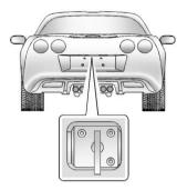
• From outside the vehicle, use the key to open the hatch/trunk. See Keys on page 2-1.
