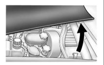
2. Go to the side of the vehicle and pull up on the rear edge of the hood, near the windshield.
