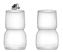
(Top Tether Anchor): Seating positions with top tether anchors.
