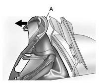
Pull the convertible top up by firmly gripping the front edge (A) near the center and applying a brisk upward and forward motion to get the top in the full-up position.
