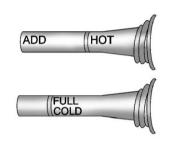
When the engine compartment is hot, the level should be at the HOT mark. When the engine compartment is cool, the level should be at the FULL COLD mark.
